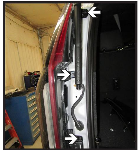
3. Using a T15 Torx, remove the three (3) bolts attaching the tail light to the vehicle.
