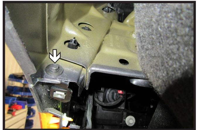
4. Pull back the wheel well liner. Using a 7MM socket, remove the one (1) bolt from the fascia joint. Do this on both sides of the vehicle.
