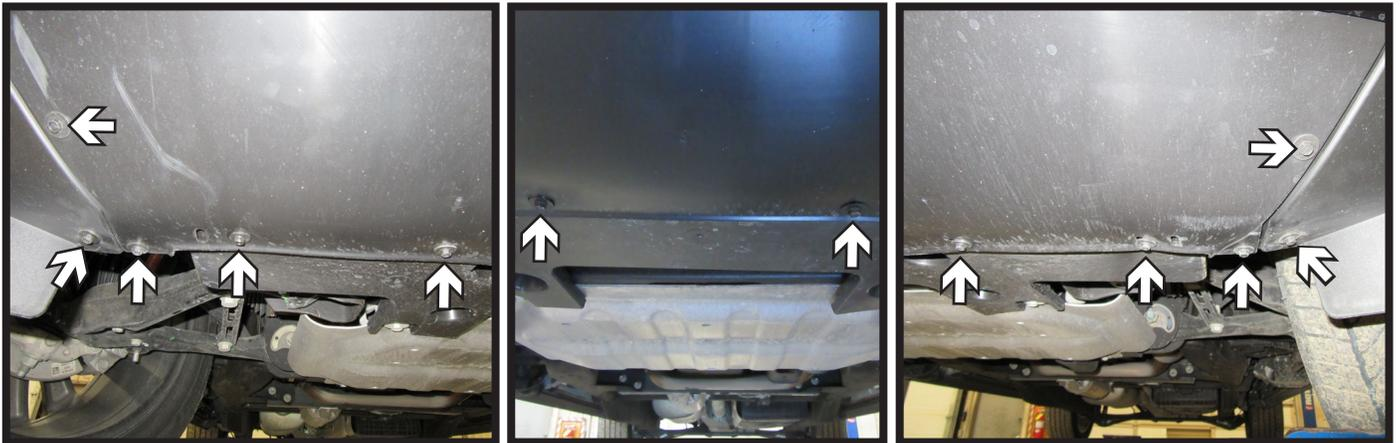
7. Using a 7MM socket, remove the twelve (12) bolts from the side and back of the skid plate.
