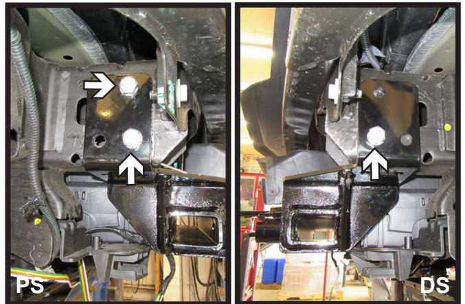
17. Slide the baseplate onto the vehicle and install three (3) 1/2" bolts with lock washers and whiz nuts, two (2) bolts on the passenger side and one (1) on the driver side.
