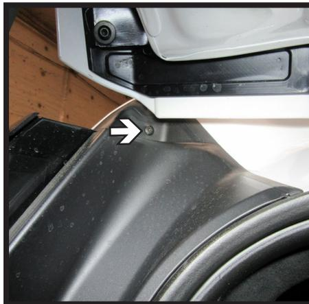
2. Using a T15 Torx, remove the one (1) bolt at the top of upper plastic cover. Remove upper cover.
