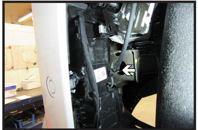
11. Disconnect washer tube on the driver side of the vehicle. Remove fascia and set aside to be reinstalled later.
