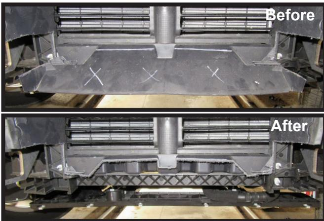
16. Using a reciprocating saw cut along the bottom back edge of the shroud as shown and remove bottom piece.
