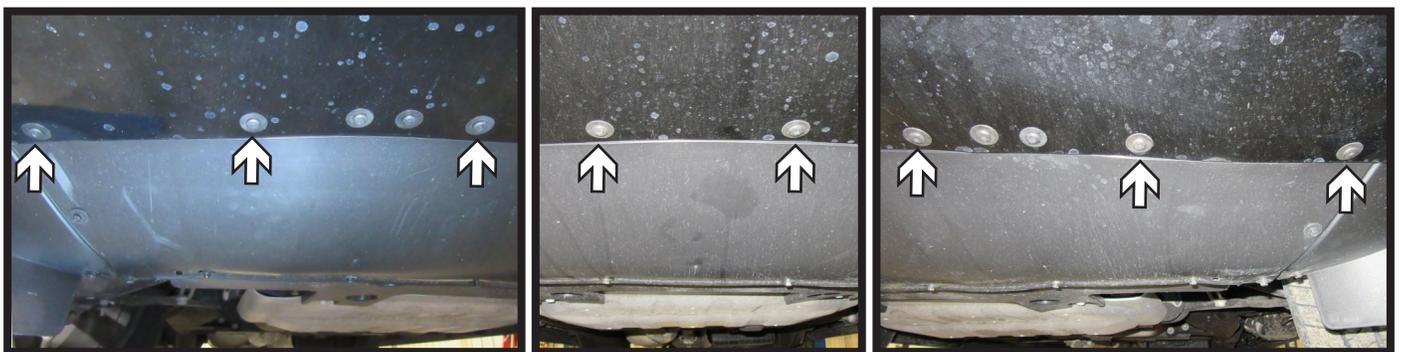
6. Using a T15 Torx, remove the eight (8) bolts from the front edge of the belly pan.
