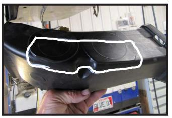
18. Hold the fascia as close to its original position, mark and trim the fascia around the convenience links and attachment tabs. Reinstall the fascia and fascia cover.
