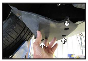
Using a Phillips screwdriver, remove three (3) screws from under the plastic piece on the outside of the vehicle. Do this for both sides of the vehicle.
