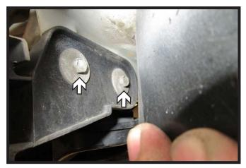
8. Under the wheel well, pull back the plastic cover. Using a 10MM socket, remove the two (bolts). Do this for both sides of the vehicle.
