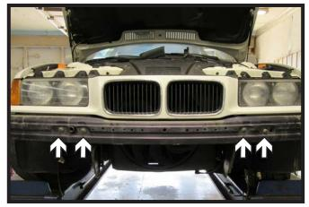
10. Using a 13MM socket, remove the four (4) bolts from the front of the bumper.
