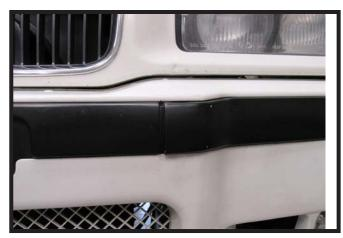
9. On the front of the car, pop the black plastic bumper off. Under the bumper, there will be three (3) push pins to be removed (removed bumper not pictured). Do this for both sides of the vehicle. Pull the corners of the fascia away from the vehicle disconnecting any electrical connections and set the fascia aside.
