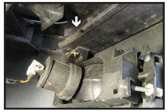
7. Using an 8MM socket, remove the screw from the top of the fascia (View from below is pictured). Do this for both sides of the vehicle.
