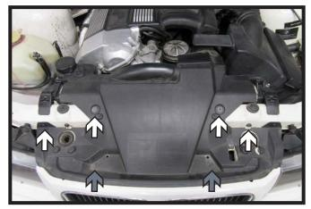
Using a T25 Torx, remove the two (2) screws from the top edge of the fascia (gray). Using a Phillips screwdriver, remove the four (4) push pins (white).
