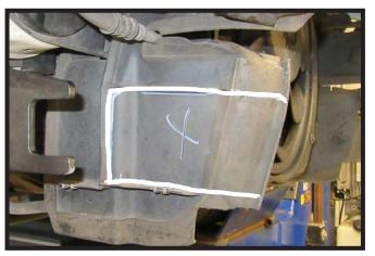
15. Using a reciprocating saw, trim the plastic shrouding approximately as shown for baseplate clearance.
