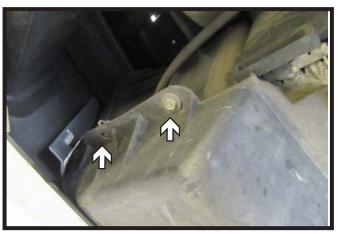
4. Using an 8MM socket, remove four (4) bolts from the belly pan of the car. There should be two (2) on each side of the pan. Remove the belly pan and set aside.
