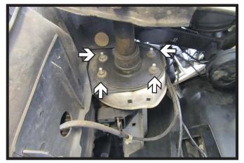
Using a 10MM socket, remove four (4) bolts from the bumper horn. Do this for both sides of the vehicle.
