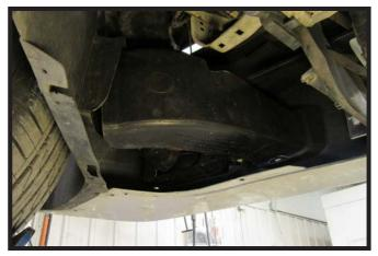
6. Underneath the car, remove the plastic air baffle by gently pulling it out. Do this for both sides of the vehicle.
