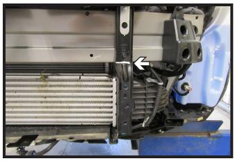
Using a reciprocating saw, trim the bracket flush with the bottom side of the bumper.
