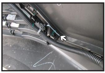
17. On the backside of the fascia, trim the lower tab back flush with the lip. Do this on both sides of the fascia.
