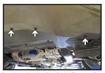
5. Using a 7MM socket, remove the ten (10) bolts from the underside of the fascia. There are five (5) on each side.
