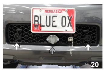
20. Align the fascia to its original position and trim the opening for the attachment tabs with a utility knife (white arrows). Do this to both sides of the vehicle. **Optional:** Attach the electrical bracket to the center of the fascia (gray arrow).
