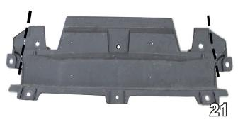
21. Reinstall the grill and fascia using the existing hardware. To reinstall the black belly pan, you have to trim the outer edges, as shown above. Tighten all bolts with Loctite Red.
