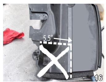
16. Using a utility knife, trim a rectangle from the black deflector 5-1/2" in from flush with the first large ridge in the back bottom corner. Do this on both sides of the vehicle.
