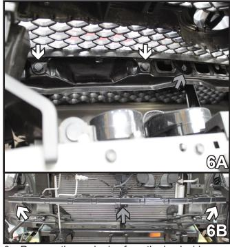
6. Remove the push pins from the back side of the grill (A, white arrows). Use a 10MM socket to remove the bolt from the center of the grill (A, gray arrow). Once the grill is off, locate the other two (2) 10MM bolts located near each headlight and remove them and the black rail (B). Remove fascia and grill then set push pins, bolts, fascia and grill aside to be reinstalled later.
