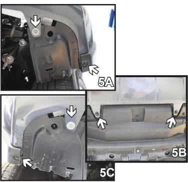
5. Starting in front of the driver's side front tire (5A), use a 10MM socket to remove the six (6) bolts from the underside (5B) of the fascia following the front bumper to the passenger's side (5C). Unplug the running and fog lights located in the center of the vehicle. Set bolts aside to be reinstalled later.
