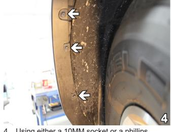
4. Using either a 10MM socket or a phillips screwdriver, remove three (3) screws located in the driver's side wheel well in front of the tire. Do this on both sides. Set screws aside to be reinstalled later.
