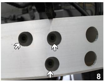
8. Use a 14MM socket to remove three (3) bolts from the front bumper on each side of the vehicle.
