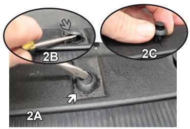
2. To remove some of the push pins, push the inner pin down until it locks with a flat screwdriver (2A, white arrow), then use the screwdriver to pry the outer pin up (2B, gray arrow). To reinstall push pins, push outer ring down until the inner pin pops back up (2C).
