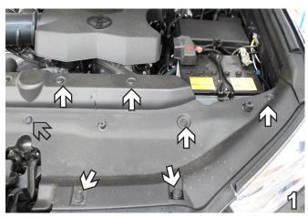
Remove six (6) push pins on both sides of the vehicle (white arrows) and one push pin from the middle (gray arrow) of the plastic cover on top of the fascia. Set push pins aside to be reinstalled later.
