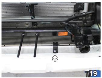
19. Optional: To install a breakaway switch, use a #10-16 x 1" self drilling screw and attach the breakaway mount to the front bumper as shown.
