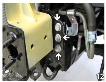
12. Using a 14MM socket, remove the three (3) bolts from the bumper bracket. Do this on both sides. Set bolts aside to be reinstalled later, and put the baseplate into position to be installed.
