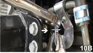
10. Using a 12MM socket, remove the bolt for the tubing bracket on each side of the vehicle (A). Then, using two pairs of large vice grips, bend the upper section of the bracket back and forth to break the top section of each bracket off (B). The bolts and removed sections will not be reinstalled.
