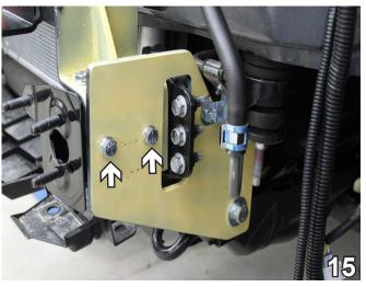
15. If necessary, use the 13/32" drill bit to clear the remaining two (2) holes in the side plate. Insert 3/8"-16 x 1-1/2" hex bolts with 3/8" lock washers and 1/4" x 1" x 1" nut plates. Do this on both sides. Use Loctite Red on all bolts.
