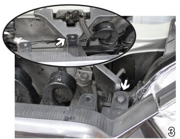
Using a 10MM socket, remove the bolt from the center of the vehicle. Use a flat screwdriver to remove a push pin from each side of the vehicle, located near each headlight. Set push pins and bolt aside to be reinstalled later.
