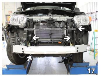
17. Reattach the black grill rail, front bumper and black plastic deflectors using the existing bolts and push pins.
