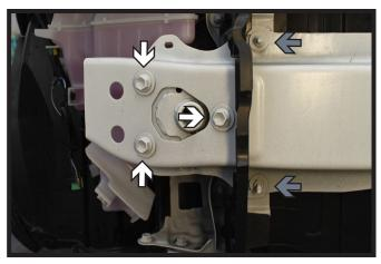
5. Using a 14MM socket, remove the six (6) bolts from the bumper. There are three (3) on each side (white).
