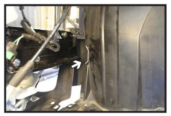
17. Notch the wheel well liner as needed around the support as shown for fascia installation. Do this on both sides of the vehicle.
