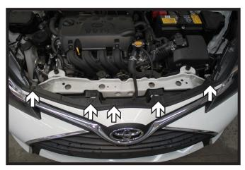
1. Remove the five (5) push pins from the top edge of the fascia.
