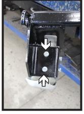
Install the frame extension onto the baseplate using the existing holes (left).
