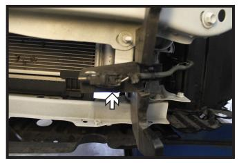
Disconnect the temperature sensor and set aside. The sensor will be relocated after baseplate installation.
