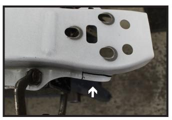
10. On the bottom side of the bumper, trim off the lower lip as shown for baseplate clearance. Do this on both sides of the bumper.
