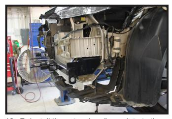
12. Reinstall the extensions/baseplate to the vehicle.
