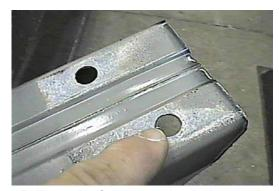
10. Drill out the four mounting holes on the back side of metal bumper with a 13/32 drill bit. Install items 6, 7, and 8 with metal bumper and tighten all bolts. Be sure and use loctite on all bolts before tightening.
