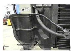
**6.** Remove two push pins on the air dam, both sides and set aside.
