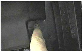
8. Remove vacuum tank from drivers side with a 10MM socket and pull out of the way.
