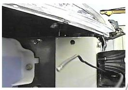
**12.** Drill remaining holes with 13/32 drill bit on the end plates. Use items 3, 4, and 5 according to drawing on last page. Reinstall end caps on metal bumper.
