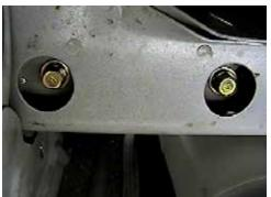
**10.** Remove two metric bolts from the bottom of frame with the 12MM socket on both sides, pull metal bumper forward and set aside.
