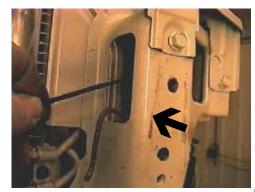
Drill out existing hole and drill all the way through to the back side of radiator cross member, both sides.
