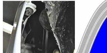
6. Pull wheel well cover back to remove metric bolt from fascia's top corner with the 10MM socket.
