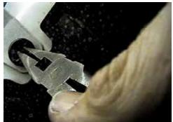
**8.** Remove two push pins from tabs on lower fascia's edge using the needle nose pliers.
