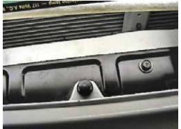
**1.** Remove two metric bolts and two push pins from the top side of fascia tabs and one metric bolt by hood latch, using the 10MM socket.
