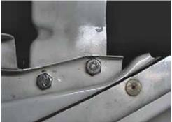
11. Drill one hole in bumper bracket on top of frame, one in bumper bracket and webbing. Insert 3/8" hex nut and lock washer into frame opening to align with drilled hole and tighten 3/8-16 x 1 bolt. Align 3/8" hex nut and lock washer with hole on the bottom side of webbing, tighten 3/8-16 x 1" bolt. Be sure and use loctite on all bolts before tightening. Torque all bolts according to the torque chart in the General Instruction sheet.
