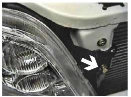
**3.** Just inside headlight assembly is one metric bolt to remove with the 10MM socket, both sides.
