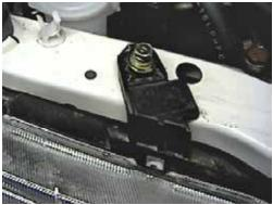
**4.** Remove two metric bolts from the top side of headlight assemblies with the 10MM socket, pull assemblies forward, unplug electrical connections and set aside.
