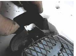
**16.** Lay fascia face down on a soft surface and trim off the back side of the lower grill with the utility knife, as shown in photo, both sides.
