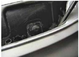
**2.** Using the flat screw driver, pull top fascia's edge back to expose and remove two push pins that release inner fascia's brace.
