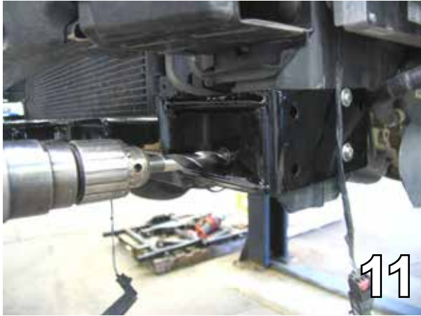
11. Using the 17/32" drill bit, drill the hole in the front of the baseplate using the baseplate as a template. Do this to both sides.
