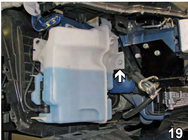
19. Reinstall the washer reservoir, on the passenger side, into the back middle hole on the baseplate. Be sure to put all the hoses and electrical connections back in place.
