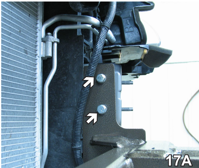
17. Install into the three drilled holes, two on the side and one on the bottom, 3/8-16 x 1 1/2" hex bolts and 3/8" lock washers with 61-5208 nut plates inserted into the frame end (photo 17B, gray arrow). Use Loctite Red on all the bolts and tighten. Do to both sides of the vehicle.
