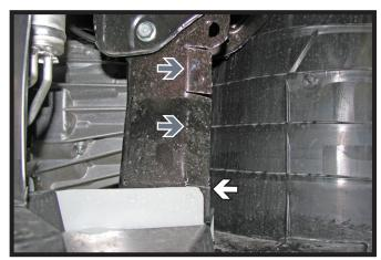
11. Using a reciprocating saw, cut the lower portion of webbing where it begins to angle down (white) to the webbing of the frame rail. Flatten the sections (above this cut, not below it) flush against the frame rail (gray) with a hammer. Do this to both sides of the vehicle.
