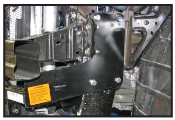
13. In the upper holes, install 3/8"-16 x 1-1/4" bolts with 3/8" lock washers, 3/8"-16 hex nuts (white). Insert one (1) 3/8"-16 nut plate through frame opening and align to lower front hole and install a 3/8"-16 x 1-1/2" bolt with 3/8" lock washer. On the driver side also include a 3/4" spacer (gray). Install 3/8"-16 x 1-1/2" bolt into the lower back hole (black) with a 3/4" spacer, 3/8" lock washer and 3/8"-16 nut. Tighten all bolts. Do this on both sides of the vehicle.
