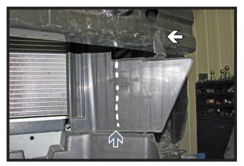
6. Remove the styrofoam reinforcement and push pin (white) from the metal bumper. Using a utility knife trim the plastic shrouding as shown (gray). Do this on both sides of the vehicle.
