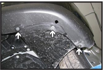
Using a 10MM socket, remove the three
