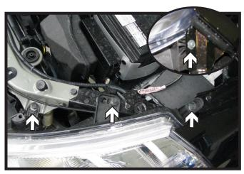
Using a 10MM socket, remove the three
