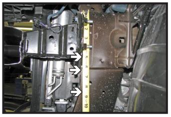
10. Mark the frame rail webbing at 5", 6-1/2" and 8-3/4" from the top of the frame rail. Using a reciprocating saw, cut the webbing to the frame rail (the top cut goes through bumper bracket also). Cut and remove the upper section of the webbing. Do this on both sides of the vehicle.
