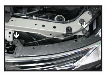
2. Remove the two (2) push pins from the top of the fascia. Do this on both sides of the vehicle.
