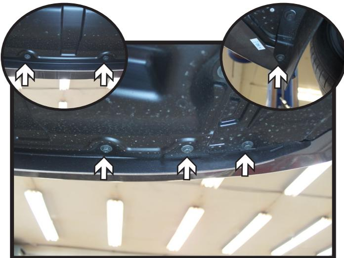
3. Using a 10MM socket, remove the ten (10) screws from the underside edge of the fascia. There are five (5) on each side of the vehicle.
