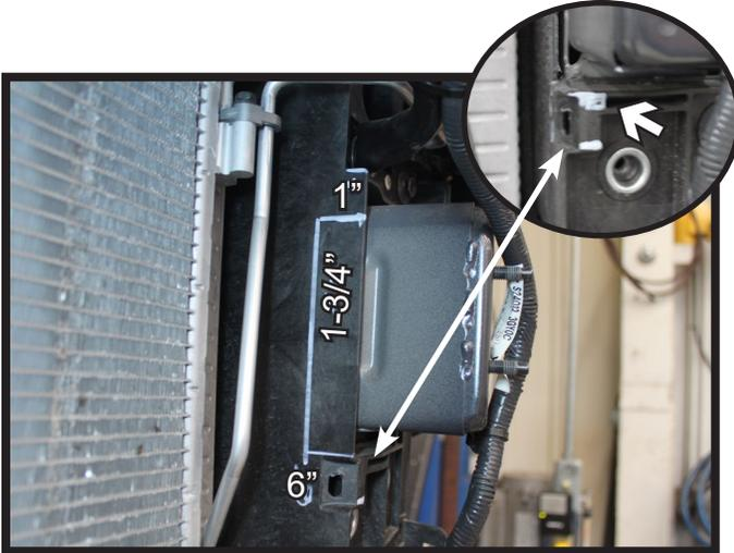
7. On the driver side, trim the plastic shielding back for baseplate clearance. Measure down 1" from the lip, back 1-3/4" and down 6".
