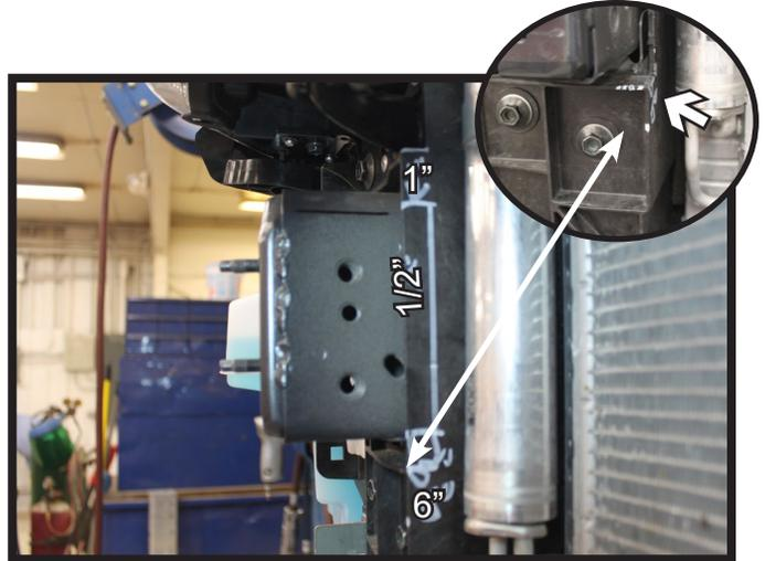
8. On the passenger side, trim the plastic shielding back for baseplate clearance. Measure down 1" from the lip, back 1/2" and down 6".
