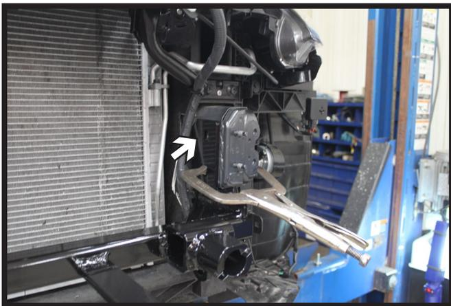
11. Using a 13/32" drill bit, drill a hole in the top front slot thru the frame on the driver side. Install a 3/8"-16 x 1-1/4" bolt with a 3/8" lock and flat washer and secure with a 3/8"-16 nut plate inside the frame. Fully tighten the bolt.
