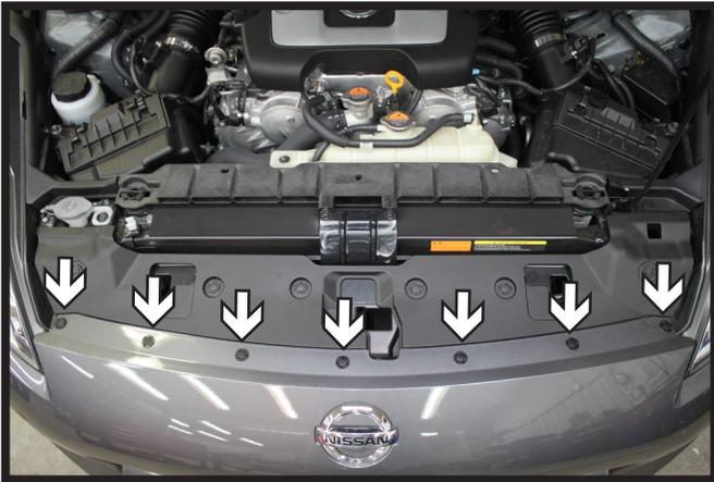
1. Remove the seven (7) push pins from the top edge of the fascia.
