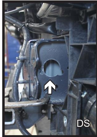
9. Using a 1-1/4" hole saw, drill an access hole on the outside of the frame on both sides of the vehicle.
