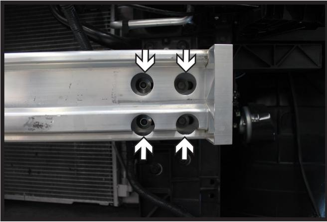
5. Using a 12MM socket, remove the eight (8) bolts from the bumper. There are four (4) on each side.
