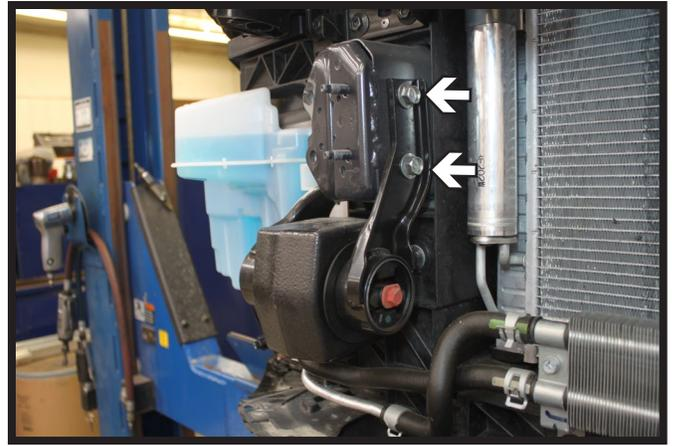
6. Using a 14MM socket and wrench, remove the two (2) bolts from the passenger side counterbalance and set aside it will not be reinstalled.
