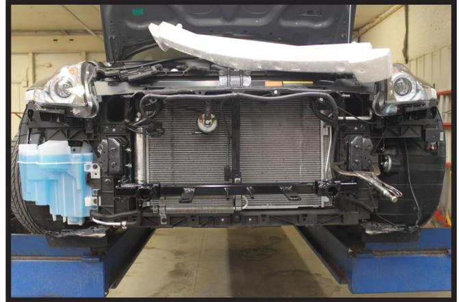
10. Position the baseplate onto the vehicle. Start the two (2) existing bolts on the passenger side, level and clamp the baseplate to the frame. Fully tighten the existing bolts.
