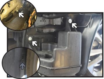
4. Using a 10MM socket, remove the three (3) screws from the air baffle. There are two (2) on the outside and one (1) on the inside of the frame (white). In the wheel well remove the push pin (gray) and set the baffle aside.
