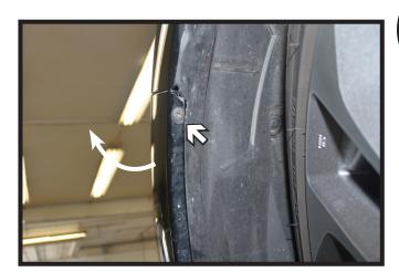
Using a Phillips screwdriver, remove the screw from the wheel well. Do this on both sides of the vehicle.
