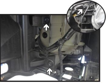
5. Remove the three (3) push pins from the shroud. There are two (2) on lower section and one (1) at the top. Unclip and remove the shroud, it will not be reinstalled. Do this on both sides of the vehicle.
