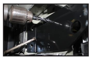
9. Position the baseplate onto the vehicle. Level and clamp the baseplate to the frame. Using a 13/32" drill bit, drill the front top hole in the baseplate thru the frame. Install a 3/8"-16 x 1-1/2" bolt with a 3/8" lock washer into the hole and secure with a 3/8" nut plate on the inside of the frame. Do this on both sides of the vehicle. Fully tighten both fasteners.
