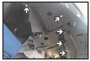
Remove the ten (10) push pins from the underside of the fascia. There are five (5) on each side.
