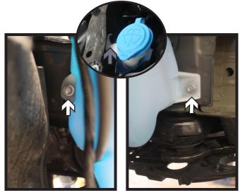
6. Using a 10MM socket, remove the two (2) screws from washer reservoir (white). Remove the push pin from the filler neck next to the cap (gray). Disconnect all lines from the reservoir and set aside.
