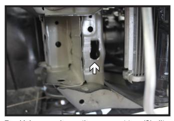
Using a reciprocating saw, cut two (2) slits vertically on the existing frame hole. Bend the tab inwards to allow nut plate access. Do this on both sides of the vehicle.
