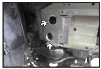
8. Using a 1-1/4" hole saw, drill two (2) access holes in the side of the frame as shown for nut plate access. Do this on both sides of the vehicle.
