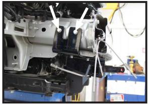
10. Using a 13/32" drill bit, drill the top two (2) holes.
