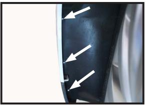
2. Using a 5.5MM socket, remove the three (3) bolts in the wheel well area. Do this on both sides.
