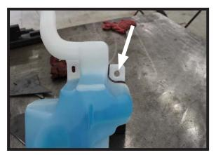
15 . Prior to reinstalling the windshield wiper reservoir, notch as shown above.
