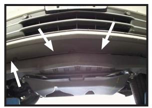
On the underside of the vehicle use a 5.5MM socket to remove seven (7) bolts. There are three (3) on per side and one (1) in the center.
