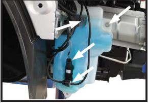
6. The windshield wiper fluid reservoir needs to be removed on the passenger side. Unplug all electrical components and remove the bolt on the top, right side using a 8MM socket. Using a 10MM socket, remove the other two (2) bolts.
