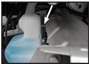
16. Place seven (7) 1/4" flat washers behind the reservoir on the inner most side prior to tightening the existing bolts.
