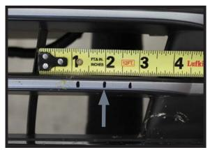
13. On the fascia measure from the outside edge (gray arrow) inward 2" and mark. On both sides of the 2" mark, measure outward 3/4".
