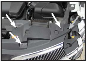
Using a 10MM socket, remove the six (6) bolts that are located in the front area, three (3) per side. There is one (1) push pin located on each side that will need to be removed also. NOTE: The bolt on the outer edge is not installed on 2012 models.
