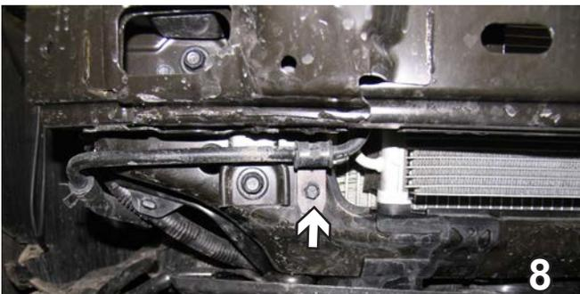
8. On the passenger side, using a 10MM socket, remove one metric bolt located underneath the metal bumper on the passenger side of the vehicle. Set bolt aside to be reinstalled later.
