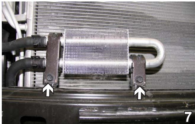
7. Using a 10MM socket, remove two metric bolts from the cooling condenser located on the passenger side of the vehicle. Please discard the bolts, because they will not be reinstalled later.
