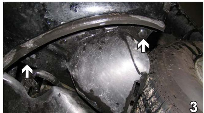
3. Using a Phillips screwdriver, remove two plastic Phillips push pins from just forward the front tire underneath. Do this to both sides of the vehicle. Set push pins aside to be reinstalled later.
