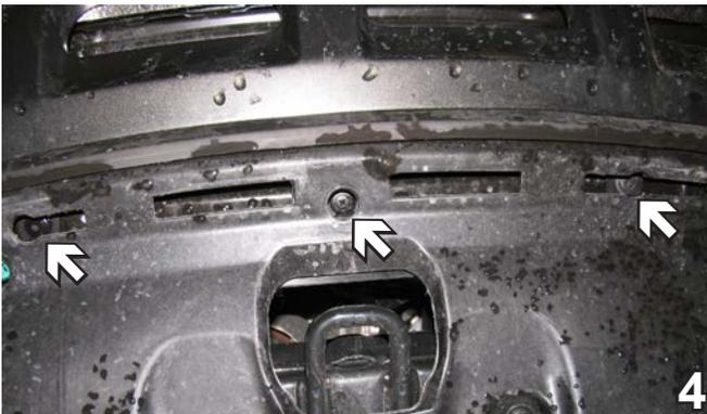
4. Using a Phillips screwdriver, remove three plastic Phillips push pins located in the middle underneath. The fascia is then ready to be removed from the vehicle. Set fascia and push pins aside carefully to be reinstalled later.
