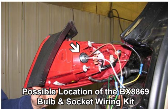
Handling of some cosmetic parts when installing this product may require the use of protective covers, rags, specialty tools, etc. to prevent damage.
