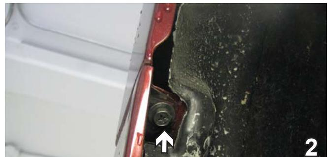
2. Using a Phillips screwdriver, remove one metric bolt just forward of the front tire, on wheel well. Do this to both sides of the vehicle. Set bolts aside to be reinstalled later.
