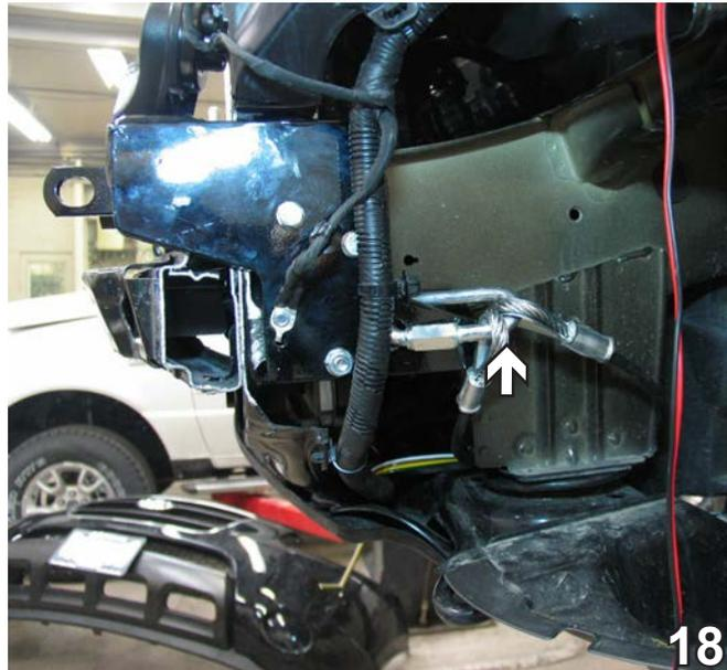
18. Attach the permanent baseplate safety cables to the provided convenience link on the baseplate. The photo above shows the recommended installation of the cables to frame of vehicle. Additional options may interfere with suggested mounting; in this case secure the cables to a solid piece of the frame as described in the instructions included with the permanent baseplate safety cables. Be sure the safety cables do not rub against any hoses or moving parts. Do this to both sides of the vehicle
