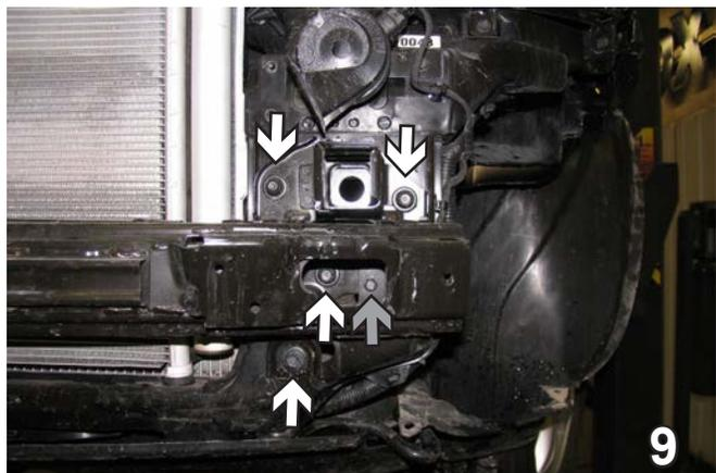
9. Using a 12MM socket, remove four metric bolts from the metal bumper (see white arrows) and then using a 10MM socket, remove one metric bolt from the inside of the metal bumper (see grey arrow). Do this to both sides of the vehicle. Set metal bumper and bolts aside to be reinstalled later.
