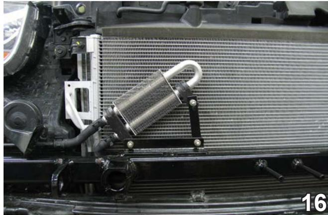
16. Reposition coolant line according to the photo above by using a condenser support and then tightening is down with 1/4-20 x 3/4" hex bolts and 1/4-20 hex flange whiz lock nuts.
