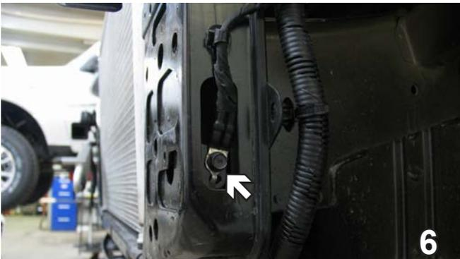
6. Using a 10MM socket, remove one bolt and release the clip from the wire harness, so it can be moved out of the way. Do this to both sides of the vehicle. Set bolts aside to be reinstalled later.
