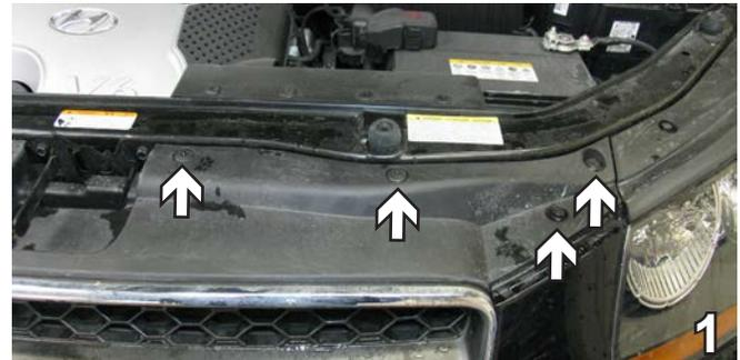
1. Using a Phillips screwdriver, remove three plastic Phillips push pins and then using a 10MM socket, remove one metric bolt. They are all located on the top edge of the fascia on the black plastic piece. Do this to both sides of the vehicle. Set push pins and bolts aside to be reinstalled later.
