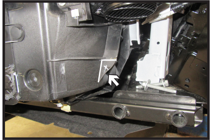
11. On the driver side of the vehicle, notch the plastic piece as shown for baseplate clearance.
