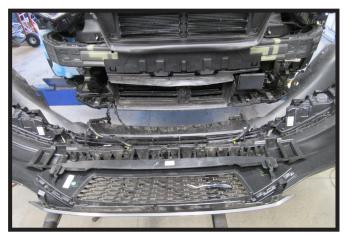
8. Pull the corners of the fascia away from the vehicle disconnecting any electrical connections and set the fascia aside.
