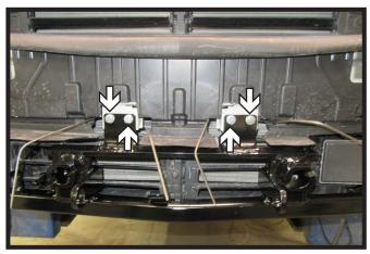
13. Slide the baseplate onto the vehicle, lining up the four bracket holes. Install four (4) 3/8" bolts with lock washers and nut plates.
