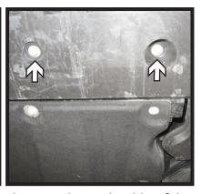
6. Using a 10MM socket, remove the eight (8) bolts from the plastic piece on the underside of the vehicle. Set piece aside to be reinstalled later.
