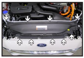
1. Remove nine (9) push pins from the fascia cover. Remove fascia cover and set aside to be reinstalled later.
