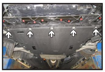
Using a 10MM socket, remove the five (5) bolts from the front edge of the belly pan. Let belly pan hang loose.
