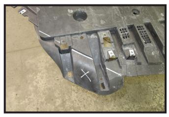
19. Using a reciprocating saw, trim the plastic piece from the underside of the vehicle as indicate. Trim the same area on both sides of the plastic piece.
