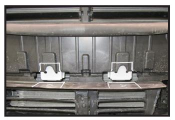
11. Using a utility knife, remove the marked areas above the shutters. (The top picture is the before and the bottom picture is the after.)
