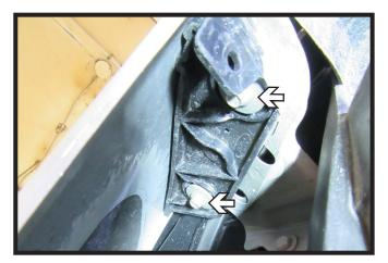
7. In front of the tire, pull back the wheel well cover. Using an 8MM socket, remove the two (2) bolts. Do this for both sides of the vehicle.
