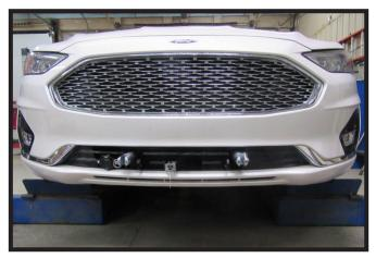
21. Hold the fascia as close to its original position, mark and trim the fascia around the convenience links, attachment tabs and electrical rods. Make sure to only trim as little as necessary to allow for tabs. The ACC unit on the driver side may malfunction if too much plastic is cut away. **Important:** Ensure that nothing is installed in front of the ACC sensor. Obstructions will cause false readings from the sensor.
