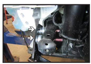
15. Insert two (2) 1/2" x 4" bolts with two (2) 1/4" spacers in between the baseplate and frame extension. Do this on both sides of the vehicle.
