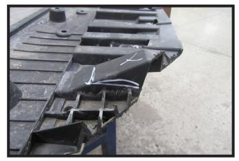
20. Flip the plastic piece over and using a reciprocating saw, trim the area as indicated on both sides of the piece.
