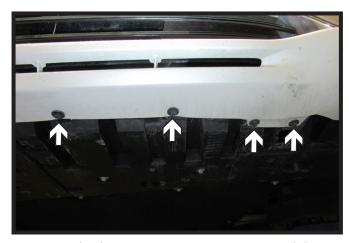
4. Underneath the car, using a 7MM socket, remove twelve (12) bolts total. There are two (2) on each side, and eight (8) along the front. (Driver's side and front pictured)
