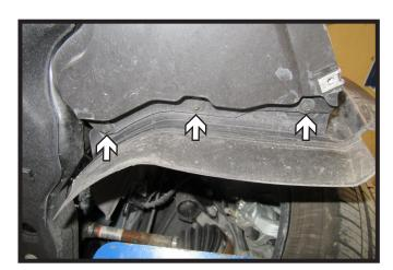
5. Using a 7MM socket remove the three (3) bolts in front of the tire on both sides of the vehicle.
