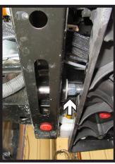
17. Insert one (1) 1/2" x 3-1/2" bolt with flat washer through existing hole from the backside of the frame and into back hole of bracket (left). Attach using second flat washer and nylon lock nut (right). Do this on both sides of the vehicle.
