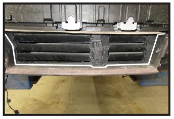
10. Using a utility knife, trim and remove the sides and bottom of the shutter housing as shown.
