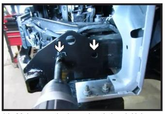
14. Make sure the baseplate is level. Using a 1/2" drill bit, drill the bottom two holes on the side plate completely through the frame using the baseplate as a template. Do this on both sides of the vehicle.
