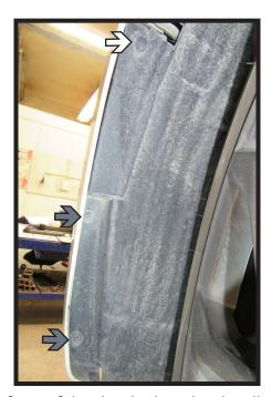
3. In front of the tire, in the wheel well, remove one (1) push pin (white). Using an 7MM socket, remove two (2) bolts (gray). Do this for both sides of the vehicle.
