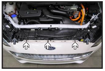
2. Using a 10MM socket, remove three (3) bolts (white) from the top of the fascia, and two (2) bolts (gray) from the plastic covers.
