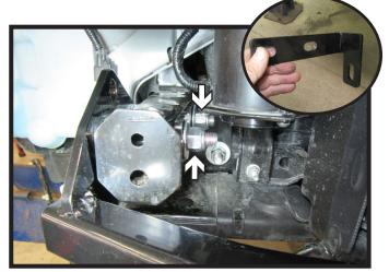
16. Place bracket (inset) on side plate 1/2" bolts with the bent portion towards the back facing downward. Attach bracket to the 1/2" bolts using a flat washer and nylon lock nut. Do this on both sides of the vehicle.
