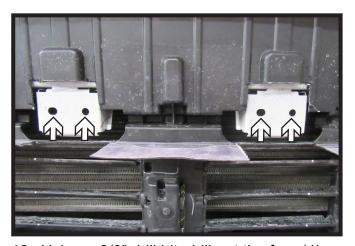
12. Using a 3/8" drill bit, drill out the four (4) holes above the shutter housing.
