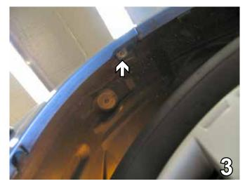
Using a Phillips screwdriver, remove Phillips screw from fascia corner just above front tire in wheel well. Do this to both sides of the vehicle, the driver's side is shown. Set these screws aside to be reinstalled later.
