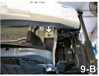
9. Using a 12MMsocke remove two metric bolts from the bumper bracket between headlight assembly and the top of the metal bumper. Do this to both sides of the vehicle (9-A shows driver's sides bumper bracket). Remove the metric bolt from the bottom bumper bracket with 12MM socket. Do this to both sides of the vehicle, lift metal bumper up to release bracket tabs. Pull bumper forward and set aside (9-B).
