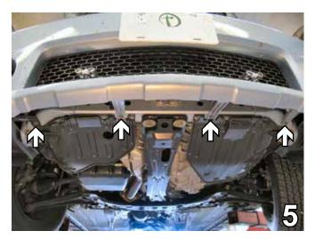
5. Using a 7MM socket, remove four metric bolts just forward of the front tire on the bottom side of fascia. Set bolts aside to be reinstalled later.
