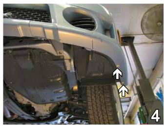
4. Forward of the front tires, on bottom edge of fascia, are two Phillips screws to remove with a Phillips screw driver. Do this to both sides of the vehicle, the driver's side is shown. Set screws aside to be reinstalled later.
