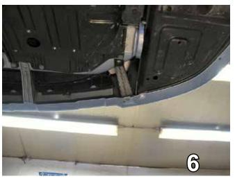
6. Using the Phillips screw driver, remove the two Phillips screws below the fascia (the passenger's side is shown).
