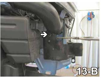
13. Slide the baseplate on the outside of tie down support where webbing was cut and align driver's side of baseplate with existing hole for front washer reservoir bolt location. Install existing reservoir bolt on driver's side, to hold baseplate in place as indicated in 13-A. Align the top middle hole of baseplate on the passenger's side with the existing hole in frame for air intake tube and clamp in place with the vise grip as indicated by 13-B. This will prepare the baseplate for drilling.
