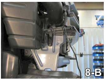
8. Remove the push pin from air intake tube on the passenger's side (8-A). Remove the two push pins from the air dam on the bottom of the metal bumper on passenger's side and one push pin on the side of the frame rail (8-B). Set push pins and air dam aside to be reinstalled later.
