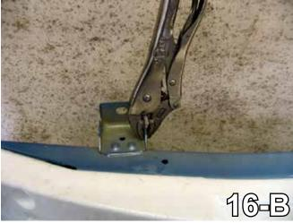
16. Set metal bumper upside down on bench, as shown in 16-A. Cut inside webbing with a reciprocating saw. Do this to both sides of the vehicle. Using he vise grips, bend webbing flat with the bottom of metal bumper see 16-B. Do this to both sides of the vehicle.
