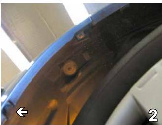
Remove one push pin from the edge of the fascia just forward of the front tire. Do this to both sides, the driver's side is shown. Set push pins aside to be reinstalled later.
