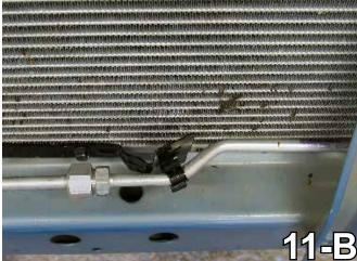
11. Behind the bracket for sensor toward radiator as shown in 11-A. This will allow the condenser tube to be moved closer to radiator and prepare the area for baseplate installation. Reinstall the temperature sensor.
