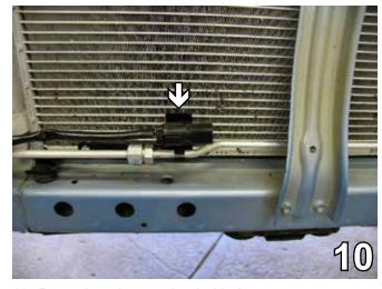
Press the tabs together behind temperature sensor bracket to release sensor and set senor up out of the way to be reinstalled later. When using power drills be aware of the dangers of torque and drill bit length.
