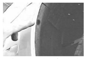
2. Remove the push pins from the wheel well molding forward of the tires.
