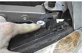
3. Remove two 10MM bolts, each side from head light fixture, unplug, and pull forward. Set light fixture aside.
