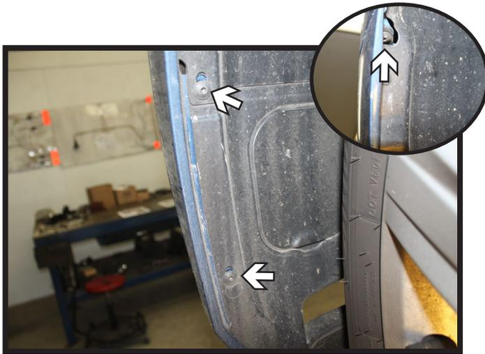
3. Using a T25 Torx, remove the three (3) screws from the wheel well. There are two (2) along the edge and one (1) at the fascia joint (inset). Do this on both sides of the vehicle.
