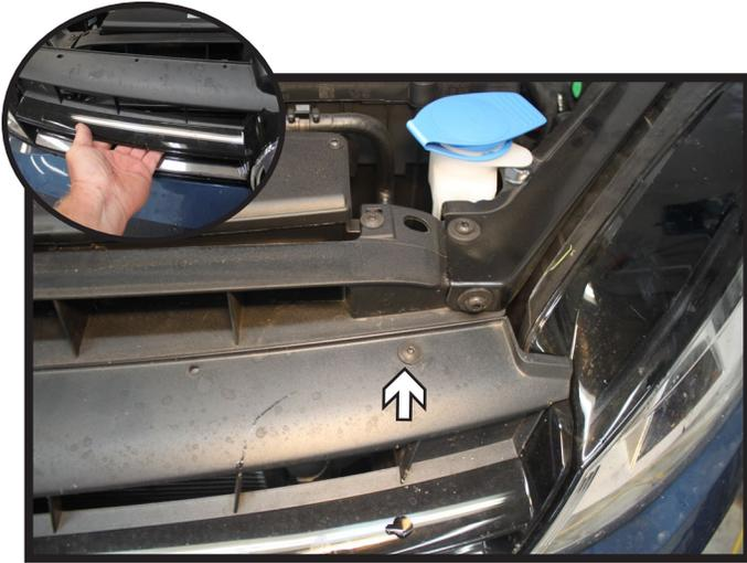
1. Using a T25 Torx, remove the two (2) screws from the top edge of the grille. There is one (1) on each side. Unsnap the grille from the vehicle and set aside.
