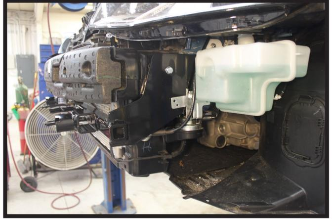
16. Reinstall the washer reservoir, temperature sensor and styrofoam support.
