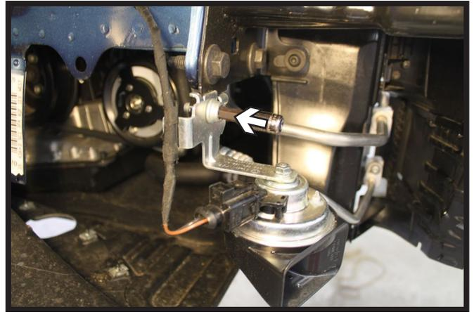
6. Using a 5/16" Allen socket or wrench, remove the screw from the horn bracket and set the horn assembly aside. Do this on both sides of the vehicle.
