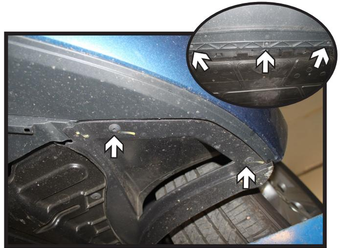
4. Using a T25 Torx, remove the seven (7) screws from the underside of the fascia. There are two (2) on each side in each corner and three (3) across the middle. Remove the fascia from the vehicle, disconnecting any electrical connections and set aside.
