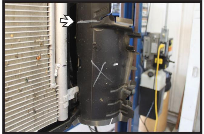
9. Trim the plastic shielding just below the notch as shown. Do this on both sides of the vehicle.
