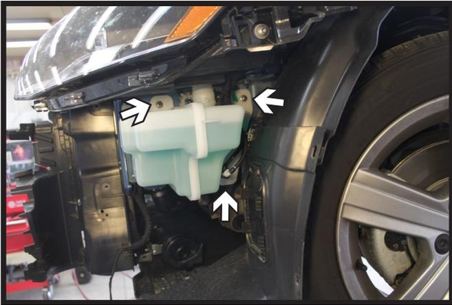
8. Using a 10MM socket, remove the three (3) screws from the washer reservoir. Disconnect/plug all lines and set aside.
