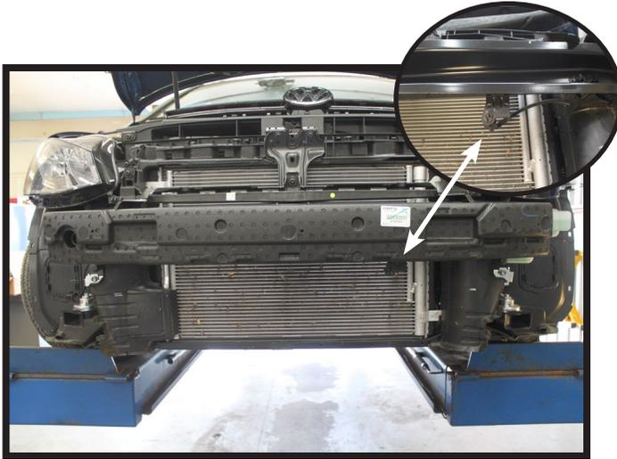
5. Remove the styrofoam support from the face of the bumper.
