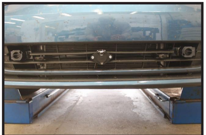
18. Hold the fascia as close to its original position, mark and trim the fascia around the convenience links and attachment tabs. Reinstall the fascia and grille.
