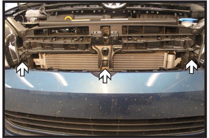
2. Using a T30 Torx, remove the three (3) screws from the top edge of the fascia.
