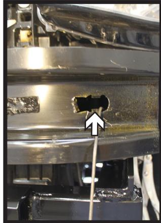
12. Using a 1-1/4" hole saw, drill an access hole on the underside of the bumper on the passenger side only (left).
