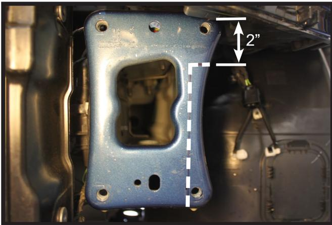
10. Using a reciprocating saw, trim the outer flange of the frame down 2" and back to the face of the frame. Do this on both sides of the vehicle.
