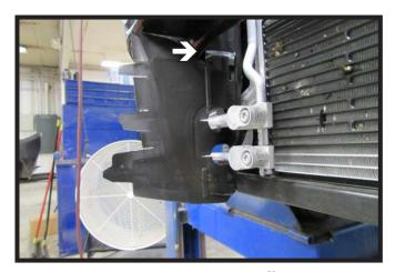
15. Trim the plastic shrouding off just below the bumper. Do this on both sides of the vehicle.
