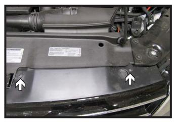
Using a T25 Torx, remove the two (2) screws from the top edge of the fascia. There are two (2) on each side.
