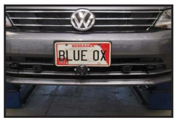
25. Reinstall the stryofoam bumper. Hold the fascia as close to its original position, mark and trim the fascia around the convenience links and attachment tabs. Reinstall the fascia.
