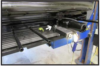
23. **Optional Breakaway:** Attach the breakaway to the baseplate with supplied 1/4"hardware.
