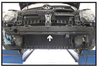
6. Remove the glued styrofoam bumper by prying gently in multiple locations.
