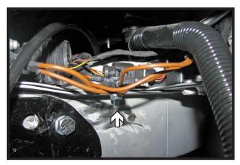
22. On the driver side, drill a 1/4" hole in the edge of the frame. Attach all the ground wires together with a 1/4"-20 x 1" bolt and 1/4"-20 lock nut.
