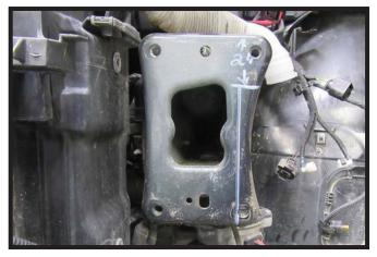
11. Using a reciprocating saw, trim the outer flange of the frame down 2" from the top and back to the face of the frame down thru the bottom lip. Do this on both sides of the vehicle.
