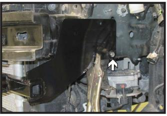
15. Position the baseplate on the vehicle so there is approximately 10-1/4" distance between the back of the baseplate and front of the bumper. Level and clamp the baseplate. Make sure that the baseplate is not hitting radiator lines or the ACC. Do this on both sides of the vehicle.
