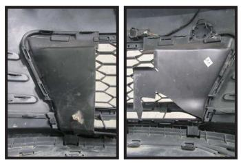
22. Before reinstalling the fascia unclip the plastic pieces on the back of the fascia and remove. These will not be reinstalled.
