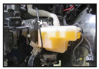
20. Reinstall the windshield washer fluid reservoir using four (4) flat washers on the top left stud in between the tank and the frame. This will space the tank so it clears the baseplate.
