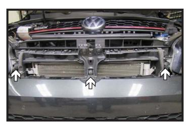
3. Using a T30 Torx, remove the three (3) bolts from the fascia brace.
