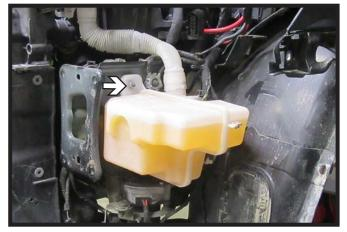
10. Using a 10MM socket, remove the three (3) nuts from the washer reservoir. Disconnect/plug all lines and set the reservoir aside to be reinstalled later.
