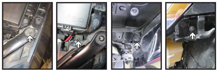
9. Using a T30 Torx, remove the four (4) bolts from the driver side headlight. There are three (3) on the top side and one (1) on the side.
