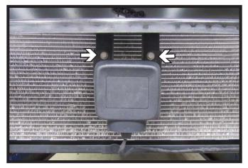
Using a 10 MM socket remove the (2) bolts attaching the Adaptive Cruise Control (ACC) to the bumper. Let hang to be reattached later.
