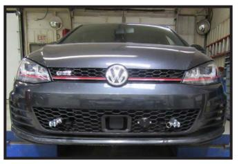
23. Hold the fascia as close to its original position, mark and trim the fascia around the convenience links and attachment tabs. Reinstall the fascia and grill.
