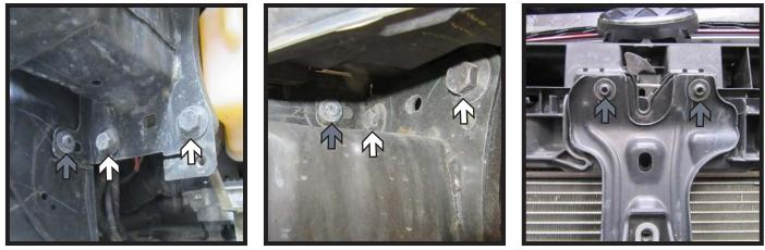
8. Using a 16MM socket, remove the eight (8) bolts from the bumper. There are four (4) on each side, two (2) on top and two (2) on bottom (white).
