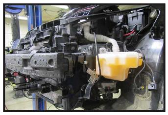
21. Reinstall the ACC, temperature sensor and styrofoam to bumper. Then reinstall the driver side head light.
