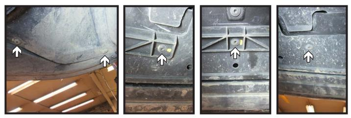
4. Using a T25 Torx, remove the seven (7) bolts from the underside of the fascia. There are two (2) on each side in each corner and three (3) across the middle.
