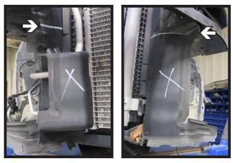
Trim the plastic shielding off just below the bumper on both sides of the vehicle. The shielding is not reinstalled.
