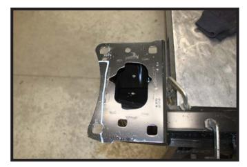
12. Temporarily reinstall the bumper. Mark the backside of the mounting flange along the cuts of the frame. Remove and trim these areas on both sides of the bumper with a reciprocating saw. Then fully reinstall the bumper and plastic fascia brace.
