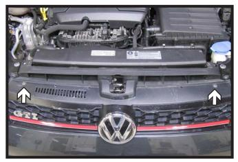
1. Using a T25 Torx, remove the two (2) bolts from the top edge of the grille. There is one (1) on each side. Unsnap the grille from the vehicle and set aside.
