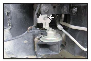
5. Using a 5/16" Allen socket or wrench, remove the screw from the horn bracket and set the horn assembly aside to be reinstalled later. Do this on both sides of the vehicle.
