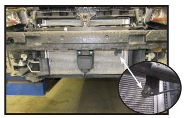
6. Remove the styrofoam support from the face of the bumper.
