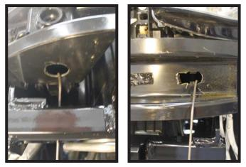
14. Using a 1-1/4" hole saw, drill an access hole on the underside of the bumper on the passenger side only (left).
