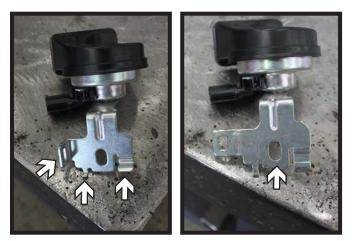
16. Prior to drilling and installing the remainder of the baseplate bolts, flatten the three (3) tabs of the horn brackets (left) so it will sit flat on the face of the side plate. Also it may be necessary to ream out the slot to accommodate the hardware (right).
