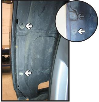
Using a T25 Torx, remove the four (4) bolts from the wheel well. There are three (3) along the edge (white) and one (1) at the fascia joint (gray). Do this on both sides of the vehicle.
