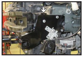
18. **Optional:** If needed a couple spacer places have been included. These can be slid down between the baseplate and the frame if there is a gap. Then tighten bolt fully.
