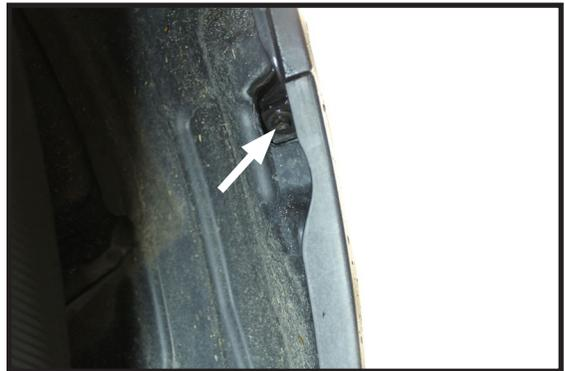
2. In the wheel well area directly ahead of the front tire towards the bottom is an 8MM bolt that needs to be removed. Further up along the trim there is a push pin that will also need to be removed in order to remove the front fascia.
