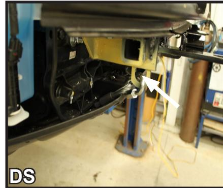
13. Attach the permanent baseplate safety cables to the provided convenience link on the baseplate. The photo above shows the recommended installation of the cables. Additional options may interfere with suggested mounting; in this case, secure the cables to a solid piece of the frame as described in the instructions included with the permanent baseplate safety cables. Be sure the safety cables do not rub against any hoses or moving parts. Do this on both sides of the vehicle.
