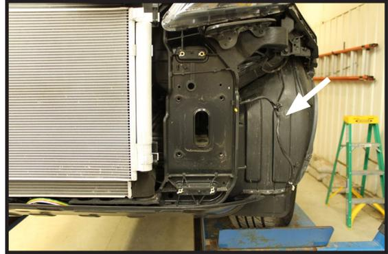
7. The temperature sensor will need to be temporarily relocated. Unclip it from the bumper and move off to the side.
