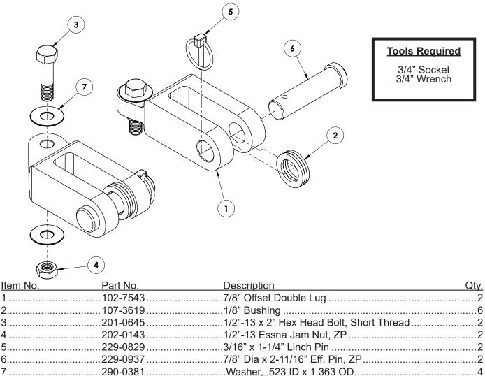
Note: If the bumper attachment plate is 7/8" thick use the supplied 1/8" spacer between the plate and lug.
