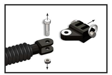
Using a 3/4" socket and wrench, remove the existing 1/2"-13 bolt and 1/2"-13 jam nut from the tow bar leg. Remove the existing lug and washers from the tow bar leg. Do this on both tow bar legs.
