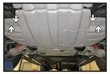
Using a 13MM socket, remove the four (4) bolts, two (2) from each side, under the tow hooks. Remove belly pan and set aside to be reinstalled later.
