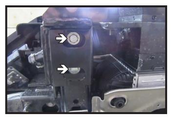
3. Slide baseplate onto tow hook housing and install two (2) 1/2" bolts with hardware into the bottom holes. Do this on both sides of the vehicle.
