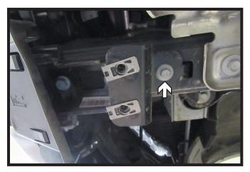
3. Using a 13MM socket, remove the one (1) bolt from the belly pan bracket. Remove bracket and set aside to be reinstalled later. Do this on both sides of the vehicle.
