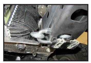
6a. Raptor & Tremor 402A Models: Attach the permanent baseplate safety cables to the provided convenience link on the baseplate. The photo above shows the recommended installation of the cables to frame of vehicle. Additional options may interfere with suggested mounting; in this case, secure the cables to a solid piece of the frame as described in the General Information sheet. Be sure the safety cables do not rub against any hoses or moving parts. Do this on BOTH sides of the vehicle.
