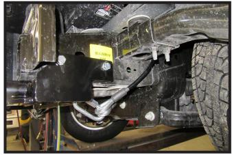
6b. All Other Models: Attach the permanent baseplate safety cables to the provided convenience link on the baseplate. The photo above shows the recommended installation of the cables to frame of vehicle. Additional options may interfere with suggested mounting; in this case, secure the cables to a solid piece of the frame as described in the General Information sheet. Be sure the safety cables do not rub against any hoses or moving parts. Do this on BOTH sides of the vehicle.
