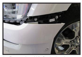
Remove the middle fascia piece by grabbing the edge and pulling outward. Set piece aside to be reinstalled later.
