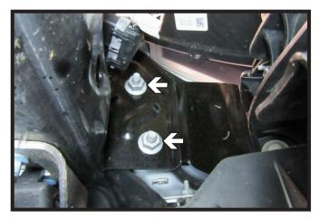
7. Coming from underneath the vehicle, use a 21MM socket to remove the two (2) outer nuts from behind the bumper. Do this on both sides of the vehicle.
