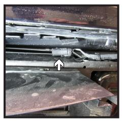
5. Start to remove the bumper. As the bumper is removed unplug the main electrical (left) and shutters (center) from passenger side of the vehicle. Then unplug electrical on top of the shutter housing (right) on the driver side of the vehicle. Set bumper aside to be reinstalled later.
