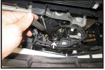
Coming from above the bumper, use a 21MM socket to remove the one (1) inside nut from behind the bumper. Do this on both sides of the vehicle.
