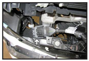
9. Unplug the main electrical on the passenger side of the vehicle.
