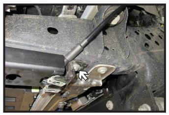
Raptor & Tremor 402A Models: Reinstall belly pan bracket before installing baseplate safety cables. Do this on both sides of the vehicle.
