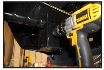
3. Using a 1/2" drill bit, ream out the lower existing hole thru the frame extension. Do this on both sides of the vehicle.
