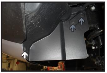
1. **Rebel Models Only:** Using an 8MM socket, remove the three (3) screws from the lower wheel well liner (white). Then remove the two (2) push pins (gray) and set the liner aside. Do this on both sides of the vehicle.
