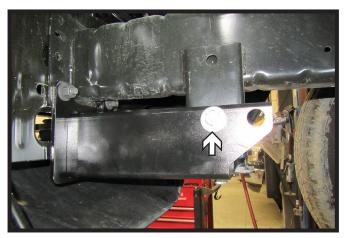
Install the 1/2" bolt with hardware into the rear baseplate hole thru the extension.
