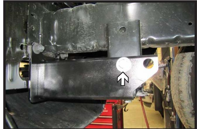
5. Install the 1/2" bolt with hardware into the rear baseplate hole thru the extension. Fully tighten all hardware. Do this on both sides of the vehicle.
