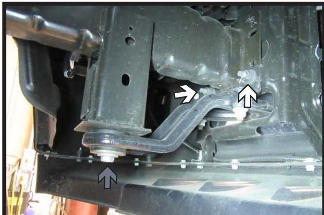
2. Using an 18MM socket, remove the two (2) nuts (white) and one (1) bolt (gray) from the tow hook and set aside. Do this on both sides of the vehicle. The tow hooks will not be reinstalled, but the hardware will be reused.
