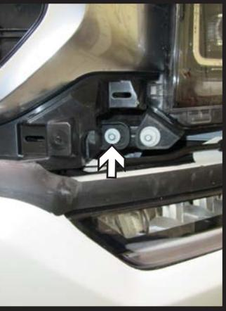
5. Using an 8MM socket, remove the two (2) inside bolts, one (1) on each side of the vehicle.
