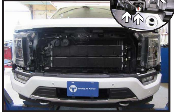
6. Lift the fascia cover and unplug the electrical connections (inset). Remove fascia and set aside to be reinstalled later.
