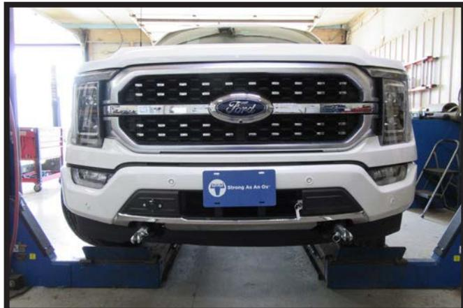
8b. **Hybrid Models:** Reinstall the bumper, fascia, fascia cover and reconnect all electrical connections.
