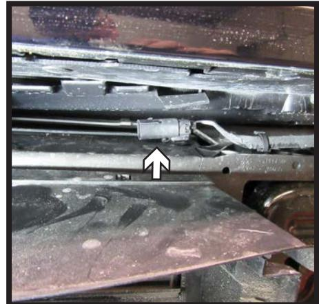
5. Start to remove the bumper. As the bumper is removed unplug the main electrical (left) and shutters (center) from passenger side of the vehicle. Then unplug electrical on top of the shutter housing (right) on the driver side of the vehicle. Set bumper aside to be reinstalled later.
