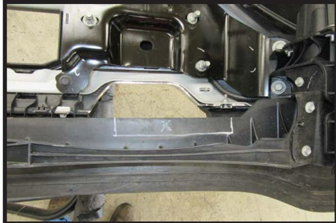
7. **Hybrid Models:** On the backside of the fascia, trim the plastic behind the tow hook opening to allow clearance for the baseplate. Do this on both sides of the vehicle.
