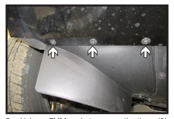
5. Using a 7MM socket, remove the three (3) bolts from the underside of the fascia in front of the tire. Do this on both sides of the vehicle.
