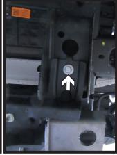
15. Using a 10MM socket, remove the two (2) bolts from the underside of the mounting bracket. Remove bracket and set aside to be reinstalled later.
