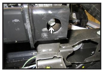
19. Using a 1/2" drill bit, drill the bottom hole on each side of the baseplate. Then install two (2) 1/2" bolts with lock nuts and whiz nuts, one (1) on each side.
