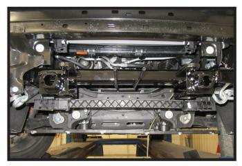
22. Reinstall the belly pan mounting bracket.
