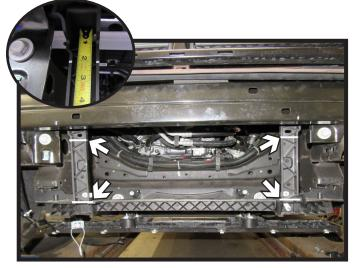
14. Using a saw, cut the two (2) vertical supports of the mounting bracket for the belly pan approximately 2" from the top (inset) and flush with the top of the lower cross member. Remove the cutout pieces.
