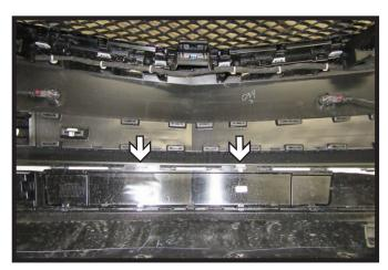
12. On the back side of the fascia, remove the two (2) white clips and pull out center piece from fascia.
