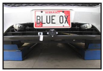
19. Hold the fascia as close to its original position, mark and trim the fascia around the convenience links and attachment tabs. Reinstall the fascia
