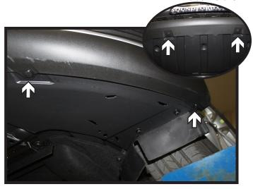
Remove the six (6) push pins from the underside of the fascia. There are two (2) in front of each wheel and two (2) in the middle.
