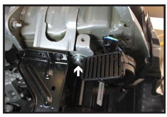
9. Using a 10MM socket, remove the screw from the passenger side horn and set the horn aside.
