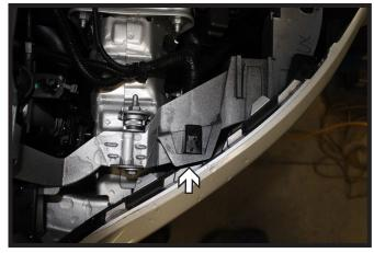
6. Release the clips underneath where the headlights were, pull the corners of the fascia away from the vehicle disconnecting any electrical connections and set the fascia aside.
