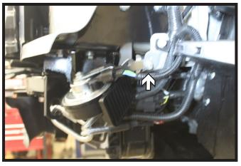
17. Bend back the webbing and reinstall the wheel well brace. Install the horn to the webbing's existing hole (white).
