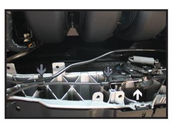
On the back side of the fascia, unhook the hood release cable from the latch (white) and unsnap the cable from the clips (gray).
