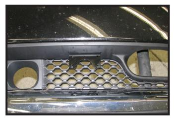
15. Install the electrical bracket to the fascia at the desired location and bent to the desired angle. With a 1/4" drill bit drill out the two (2) mounting holes thru the fascia and attach the bracket to the fascia with 1/4"-20 x 3/4" bolts and 1/4"-20 lock nuts.
