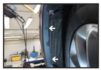
2. Using a utility knife, remove the two (2) plastic rivets from outer edge of the wheel well (white). Then using a 10MM socket, remove the upper screw (gray). Do this on both sides of the vehicle.
