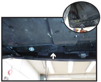
4. On the underside of the fascia, release the fascia clips by turning 90°. There is one (1) towards the middle (white) and one (1) towards the outer edge by the tire (gray). Do this on both sides of the vehicle.
