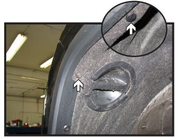
3. Along the upper edge of the wheel well, using a 10MM socket, remove the screw. Then remove the push pin further up (inset). Do this on both sides of the vehicle.
