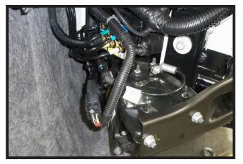
12. Loosely reinstall the compressor, checking for clearance around the baseplate. If needed shim the compressor away from the baseplate with 5/16" washers. This with keep the compressor from vibrating against the baseplate.
