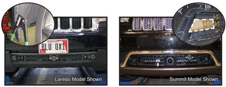
16. Hold the fascia as close to its original position as possible, mark and trim the fascia around the convenience links and attachment tabs. Reinstall the fascia. Using the plastic pop rivet gun, replace the two (2) rivets in the wheel well. Do this on both sides of the vehicle.
