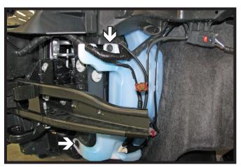
Using a 8MM socket, remove the two (2) bolts from the washer fluid reservoir. Disconnect/plug all lines and set reservoir aside.
