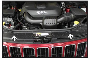
1. On the topside of the fascia, remove the two (2) push pins.
