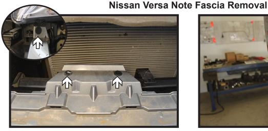
Remove the four (4) push pins from the top edge of the fascia. There are two (2) in the middle and one (1) on each side under the headlight.
