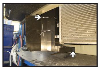
2. Trim the top part shielding as shown, remove the lower push pin and discard the shielding. Do this on both sides of the vehicle.
