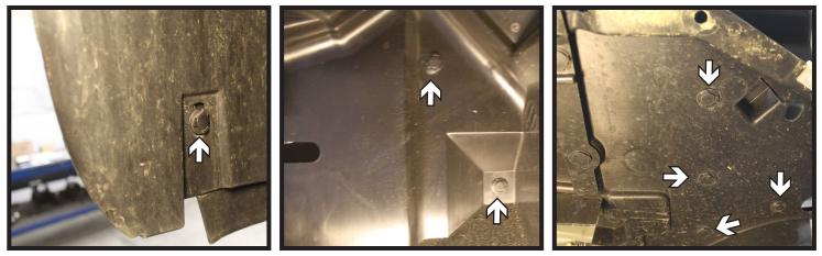
3. Remove the liner from the driver side by removing the one push pin in the wheel well (left). Then the two (2) along side the frame rail (middle) and the four (4) on the underside (right). Set the liner aside it will be reinstalled after baseplate installation.
