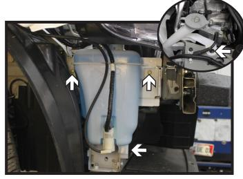
Disconnect all lines from the reservoir and plug any fluid lines. Using a 10MM socket, remove the three (3) screws from the washer reservoir.
