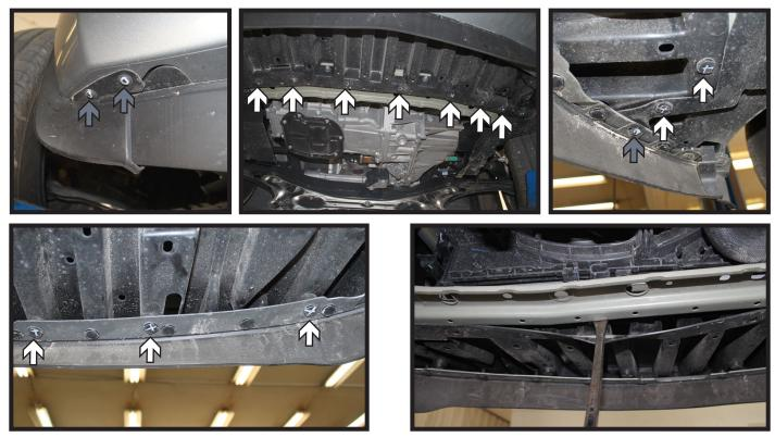
5. Remove the eighteen (18) push pins from the underside of the fascia. There are twelve (12) along the back edge of the belly pan and six (6) along the front edge. Using a T20 Torx, remove the six (6) screws (gray). There are three (3) on each side. Pry the belly pan off the studs, pull the corners of the fascia away from the vehicle disconnecting any electrical connections and set the fascia aside.
