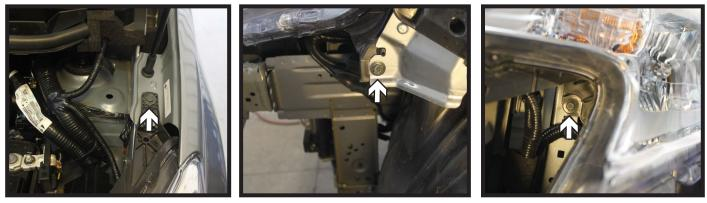
6B. **Versa Note Only:** Using a 10MM socket, remove the three (3) screws from the headlight assembly as shown. Disconnect all electrical connections and set the headlight aside. Do this on both sides of the vehicle.
