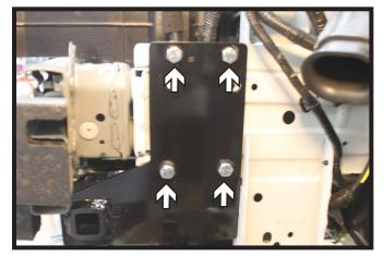
Using a 3/8" drill bit, drill the four (4) outer holes in the baseplate thru the frame. Install the 3/8" hardware and fully tighten all bolts. Do this on both sides of the vehicle.
