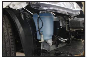
Reinstall the washer reservoir on the passenger side.
