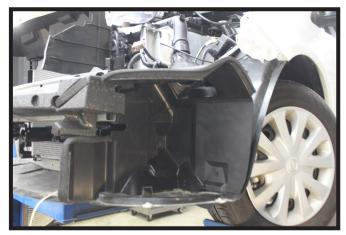
11. Reinstall the liner on the driver side.
