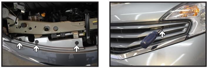
1. Remove the five (5) push pins from the top edge of the fascia. There are two (2) on the driver side and three (3) on the passenger side (left).
