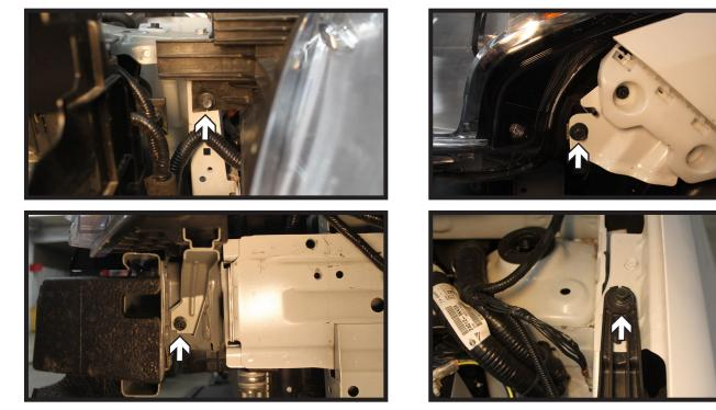
6A. **Versa Sedan Only:** Using a 10MM socket, remove the four (4) screws from the headlight assembly as shown. Disconnect all electrical connections and set the headlight aside. Do this on both sides of the vehicle.
