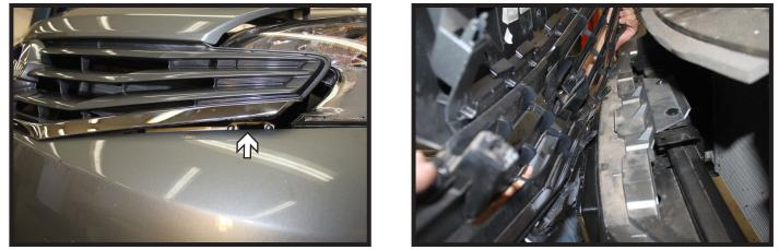
2. Remove the grille from the vehicle by unsnapping the eight (8) clips from along the backside of the grille. Set the grille aside.
