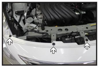
Remove the five (5) push pins from the top edge of the fascia. There are two (2) on the driver side and three (3) on the passenger side.
