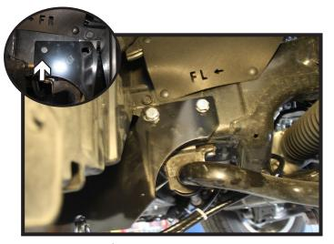
4. Using a 1/2" drill bit, drill the rear hole thru the frame (inset). Also if necessary ream the front hole with the 1/2" drill bit if the baseplate did not line up with the existing hole.
