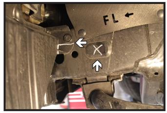
Remove the plastic plug from the frame (right). Then trim off the lower part of the plastic shielding for baseplate clearance (left). Do this on both sides of the vehicle.
