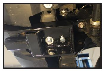
Install the baseplate onto the frame with the supplied 12MM hardware. Fully tighten all hardware. Do this on both sides of the vehicle.
