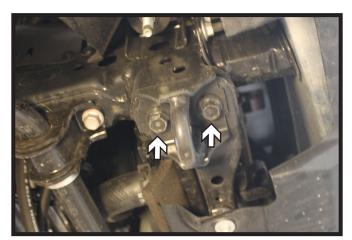
1. Using a 17MM socket, remove the two (2) bolts from the tow hook bracket. Do this on both sides of the vehicle.
