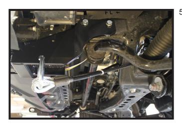
cables to the provided convenience link on the baseplate. The photo shows the recommended installation of the cables to frame of vehicle. Additional options may interfere with suggested mounting; in this case, secure the cables to a solid piece of the frame as described in the instructions included with the permanent baseplate safety cables. Be sure the safety cables do not rub against any hoses or moving parts. Do this on **BOTH** sides of the vehicle.
