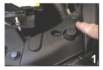
Remove the twelve pushpins from the black plastic cover on the top side of the fascia. Lift the cover and set it and the pushpins aside to be reinstalled later.
