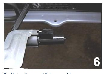
6. Using the small flat screwdriver, remove the temperature sensor and set out of the way to be reattached later.
