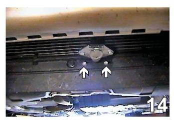
14. Using the two self tapping screws, install the electrical bracket just below the fascia on radiator cross member as shown in the photo above.
