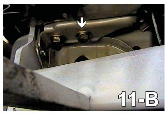
11. Using the 12MM socket, remove the two metric bolts from the top side and one from the lower side of the metal bumper just below the headlight assembly. Do this to both sides of the vehicle. Pull metal bumper forward. Set bolts and metal bumper aside to be reinstalled later.
