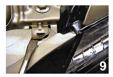
9. Using the flat screwdriver, pry up tab on the top edge of the fascia just inside of headlight assembly. Do this to both sides of the vehicle. Pull fascia's corners out to the side of the vehicle, pry fascia forward just below headlight assemblies with the flat screwdriver, pull fascia forward and set aside to be reinstalled later.
