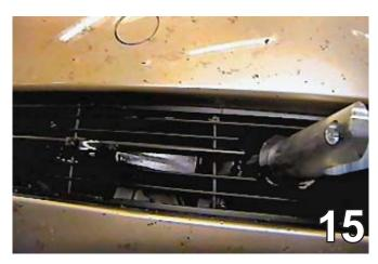
15. Hold the fascia as close to its original position as possible, trim the lower grille to allow attachment receivers to come through the lower grille and reinstall the fascia. Passenger's side is shown.
