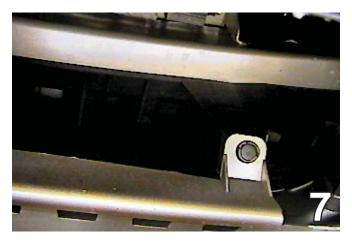
Remove two push pins from the lower edge of the front fascia, just below the license plate. Set bolts aside to be reinstalled later.
