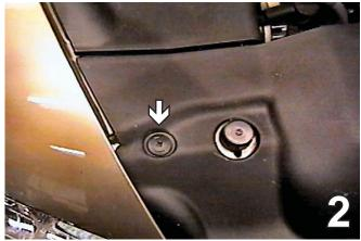
2. Remove one pushpin outside of the hood bumper. Do this to both sides of the vehicle. Lift up the black plastic cover from top side of the fascia and set aside.
