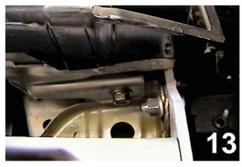
13. Reinstall the metal bumper and existing metric bolts with the 12MM socket. **NOTE:** outside metric bolt on passenger's side will not be used.
