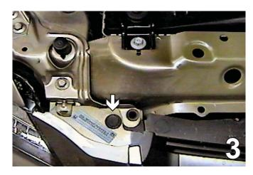
Remove the pushpin from the top edge of the fascia just inside of the headlight assembly. Do this to both sides of the vehicle.
