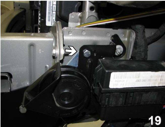
19. On the driver's side only, relocate the horn to on top of the frame with a 1/4-20 x 3/4" bolt and 1/4-20 whiz nut.
