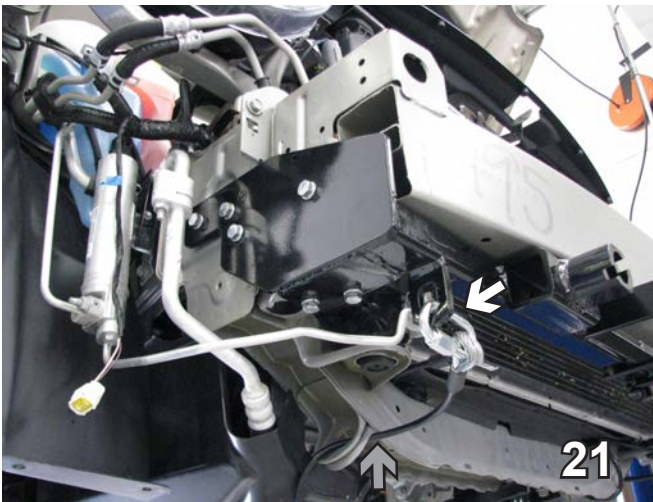
21. Attach the permanent baseplate safety cables to the provided convenience link on the baseplate (see right white arrow). The photo above shows the recommended installation of the cables to frame of vehicle (see grey arrow). Additional options may interfere with suggested mounting; in this case secure the cables to a solid piece of the frame as described in the instructions included with the permanent baseplate safety cables. Be sure the safety cables do not rub against any hoses or moving parts. Do this to both sides of the vehicle.
