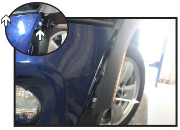
4. Pry the fender flare away from vehicle. Using a T30 Torx, remove the screw from behind the fender flare. Do this on both sides of the vehicle.
