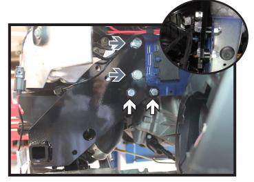
Install the baseplate to the vehicle using the existing frame holes with the supplied 12MM bolts and lock washers (gray). Level and fully tighten all bolts.
