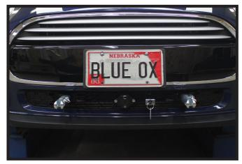
17. Hold the fascia as close to its original position, mark and trim the fascia around the convenience links and attachment tabs. Reinstall the washer reservoir and fascia
