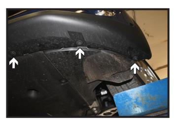
Using a 8MM socket, remove the seven (7) screws from the underside of the fascia.
