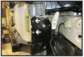
12. Using a 3/8" drill bit, drill out the front two (2) holes. Do this on both side of the vehicle.
