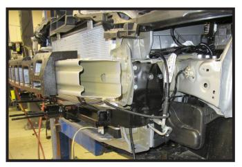
17. Reclip the temperature sensor wire loom to the baseplate. Then using a zip tie attach the sensor to the top of the baseplate.
