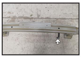
9. Remove the temperature sensor bracket from the bumper. Set aside to be relocated and reinstalled later.
