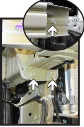
8. Using a 10MM socket remove the five (5) bolts attaching the bumper to the frame. Do this on both sides of the vehicle. Remove bumper and set aside to be reinstalled later.
