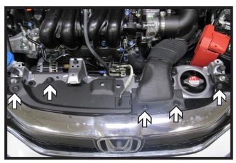
1. Remove the five (5) push pins from the fascia cover. Remove fascia cover and set aside to be reinstalled later.
