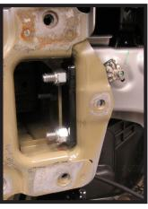
13. Install the two (2) 3/8" bolts with backing plate and nylon lock nuts on the inside. Tighten fully. Do this on both sides of the vehicle.
