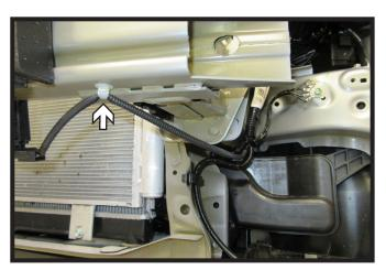
7. Unclip the temperature sensor wire loom from the bumper and unplug sensor.
