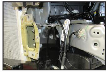
14. Remove the center bolt. Using a 3/8" drill bit, drill the final back hole. Install 3/8" bolts with backing plate and nylon lock nuts on the inside. Tighten fully. Do this on both sides of the vehicle.
