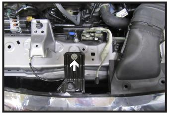
2. Using a 10MM socket to remove the one (1) bolt.
