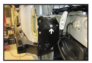
11. Using a 3/8" drill bit, drill out the center hole. Install the one (1) 3/8" bolt and hardware. Tighten but do not use Loctite® Red at this time. Do this on both sides of the vehicle.
