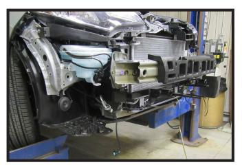
16. Reinstall the bumper on the vehicle. Then reinstall the windshield washer fluid reservoir to the passenger side of the vehicle.
