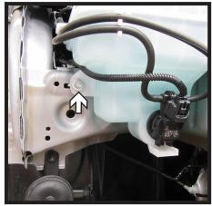
6. On the passenger side of the vehicle remove the windshield washer reservoir. Remove the one (1) push pin (gray) at the top (gray). Then using a 10MM socket remove the two (2) bolts (white) holding the reservoir. Unplug all lines, remove the reservoir and set aside to be reinstalled later.
