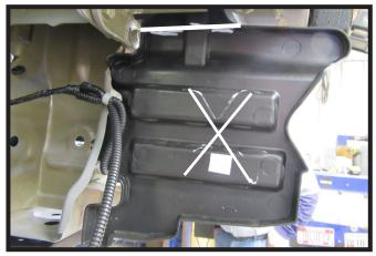
Trim plastic piece as indicated so that it is flush with the bumper. Do this on both sides of the vehicle.
