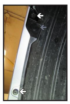
3. Using a Phillips screw driver remove the two (2) screws (white) from the wheel well. Then remove the one (1) push pin (gray).
