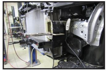
Tilt baseplate to slide into place. Make sure that the baseplate is as far upward and forward as possible. Then clamp into place.
