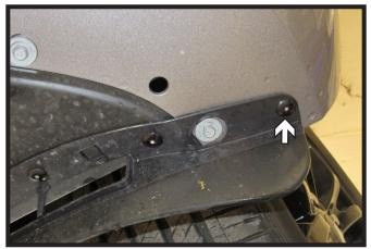
4. **Some Models**: Using a drill bit, drill out the two (2) metal rivets, there is one (1) on each side of the vehicle.
