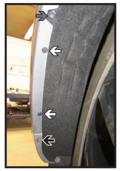
2. In the wheel well, using a 10MM socket, remove the top screw (gray). Using a 8MM socket, remove the lower screw (black). Then remove the two (2) plastic rivets (white). Do this on both sides of the vehicle.
