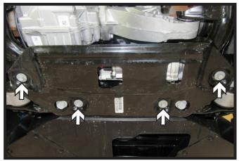
Using a 13MM socket, remove the four (4) bolts from the metal belly pan. Remove metal belly pan and set aside to be reinstalled later.
