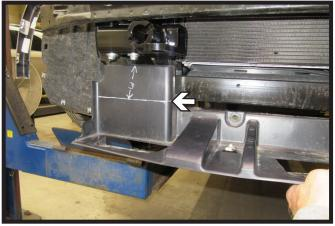
7b. **2021-2024 Models:** Hold the plastic shield up to the push pin holes and trim shield approximately 3" as shown for baseplate clearance.
