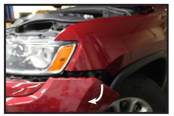
6. Pull the top corners of the fascia out releasing the clips behind, continue working inward towards the grill releasing the clips under the headlights. Pull the fascia forwards disconnecting all electrical connections and set the fascia aside to be reinstalled later.
