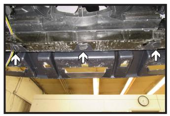
Turn the three (3) locking knobs on the bottom of the plastic shielding 90° to remove. Remove plastic shielding and set aside to be reinstalled later.
