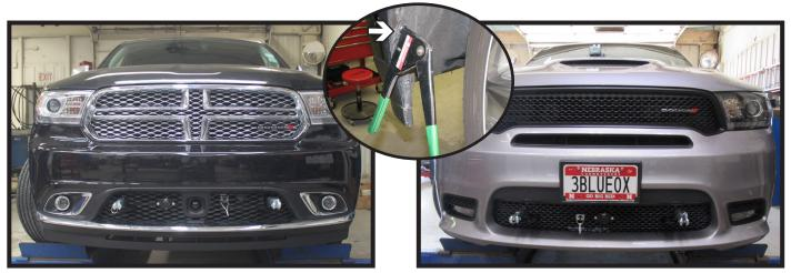
16. Hold the fascia as close to its original position, mark and trim the fascia around the convenience links and attachment tabs. Reinstall belly pan, plastic shield, fascia and reconnect all electrical connections. Using the rivet gun, replace the rivets that were removed during the fascia removal.
