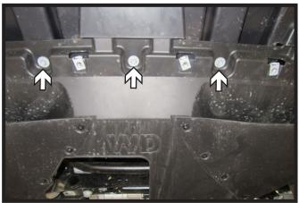
Using a 10MM socket, remove the three (3) center bolts from the front of the belly pan.
