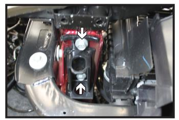
3. **Models equipped with tow hooks:** Using a 16MM socket, remove the two (2) bolts from the tow hook bracket. Remove the tow hook bracket from the vehicle. Do this on both sides of the vehicle.
