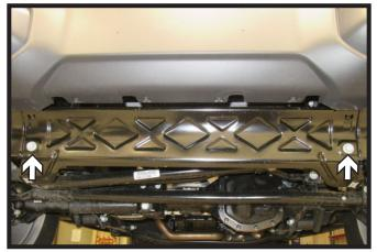
Using a 16MM socket, remove the two (2) bolts from the metal guard. Remove and set aside to be reinstalled later.
