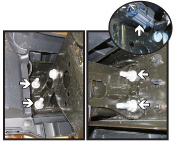
Using an 18MM socket, remove the four
