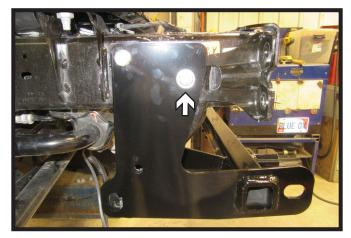
5. Remove the top front bolt and insert frame bracket between the frame and the baseplate. Make sure the bracket is flush with the front of the frame. Reinstall bolt and hardware. Do this on both sides of the vehicle.
