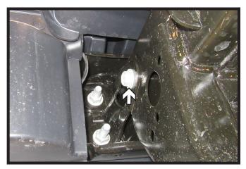
6. Using a 16MM socket, remove the one (1) bolt on the outside of the frame holding the bracket after removing the bumper. Do this on both sides of the vehicle.
