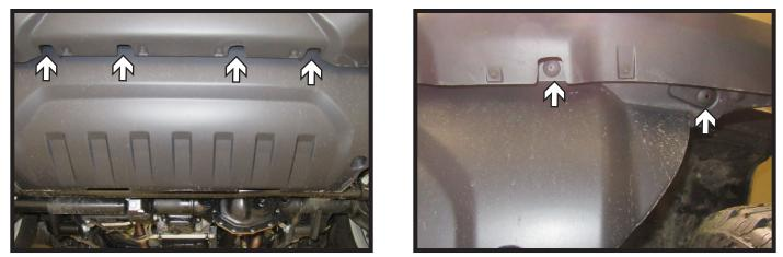
2. Remove the eight (8) push pins from the edge of the belly pan. There are four (4) in the center and two (2) on each side. Remove belly pan and set aside to be reinstalled later.
