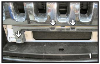
Pull the center grill insert forward to release the four clips, one on each side and two in the middle. Set insert aside to be reinstalled later. The passenger's side is shown in the photo above.
