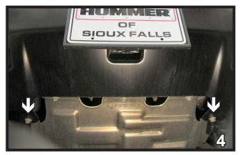
4. Just below the bumper, remove two metric bolts with the 18MM socket. Pull the metal bumper forward and disconnect the fog lights. Set bolts and metal bumper aside to be reinstalled later.
