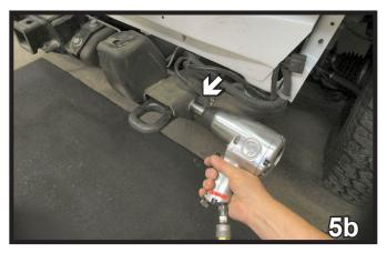
5. Using the 18MM socket, remove three metric bolts from the tow hook, two on the inside (see photo 5a) and one on the outside (see photo 5b). Pull tow hook forward and set aside. Do this to both sides of the vehicle. The tow hooks will not be reinstalled. Please return them to the customer.
