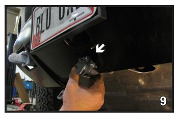
9. Using the 1" self tapping screw, install the electrical bracket just below the license plate bracket while ensuring enough clearance for the bracket cover to open.
