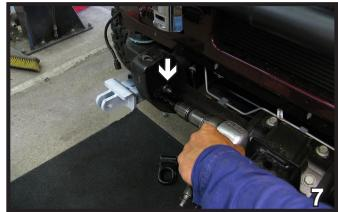
7. Using the baseplate weldment as a template, drill through the forward existing hole on the inside of the frame rail with the right angle drill and the 17/32" drill bit. Do this to both sides of the vehicle. If a right angle drill is not available, it may be necessary to remove the winch bracket to allow room for drilling.
