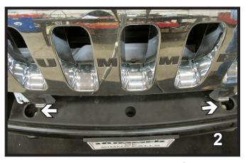
2. Remove the two rubber inserts from the top of the bumper. Set the rubber inserts aside to be reinstalled later.
