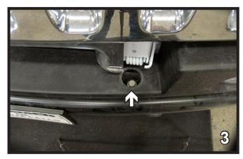
Using the 18MM socket, remove one metric bolt from the top of the bumper. Do this to both sides of the vehicle. Set bolts aside to be reinstalled later.
