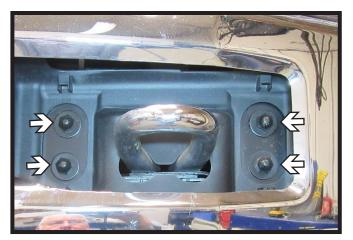
Using a 18MM socket, remove the four (4) bolts around the tow hook. Do this on both sides of the vehicle. Pull the bumper forward and set aside to be reinstalled later.
