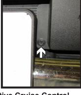
4. Models with Adaptive Cruise Control (ACC): Using a 10MM socket, remove the two (2) bolts from the cover of the ACC on the driver side of the vehicle.
