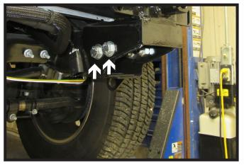
12. Use three (3) 1-3/4" bolts to attach the baseplate towards the outside of the frame. Use a flat washer on the outside and nylon lock nut on the inside for the front two (2) bolts indicated with a white arrows and a flat washer and nylon lock nut on the inside for the third bolt indicated with a gray arrow. Towards the inside of the frame use two (2) 1-3/4" bolts to attache the baseplate with the washer on the outside and nylon lock nut on the inside. Do this on both sides of the vehicle.
