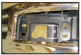
13. Using a utility knife remove the marked area on both sides of the vehicle to allow the baseplate to fit through the hole in the fascia (left). Then remove the marked area on both sides of the fascia towards the inside near the licence plate (right).
