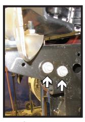
9. Remove the two (2) bolts from each side of the bracket near the tow hook by using an 18MM socket. Do this on both sides of the vehicle.
