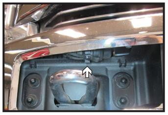
6. On the passenger side of the vehicle pull the indicated plug through the backside of the fascia and let hang.
