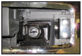
18. Trim the tow hook bolt cover as shown before reinstalling to allow room for the convenience link (left). Do this for both sides of the vehicle.
