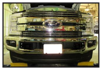
Models with ACC: Reinstall ACC and cover to the driver side of the vehicle.
