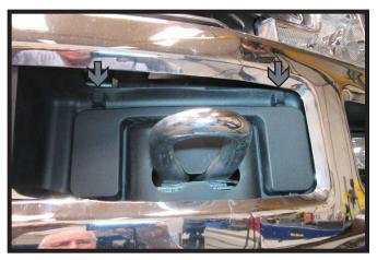
3. Remove the two (2) clips from each side above the tow hook. Do this on both sides of the vehicle.
