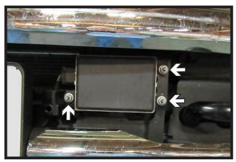
5. **Models with ACC:** Using an 11MM socket, remove the three (3) bolts holding the ACC onto the driver side of the vehicle. Unplug, remove, and set aside the ACC to be reinstalled later.
