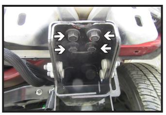
Using an 18MM socket, remove the four(4) bolts from the bottom of the tow hooks on both sides of the vehicle.
