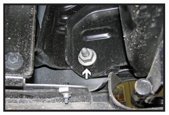
From the underside of the bumper, using a 21MM socket, remove the bolt from the outer side of the frame. Do this on both sides of the vehicle.
