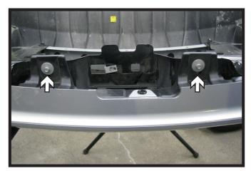
Using a 8MM socket, remove the two (2) bolts from the top side of the bumper.
