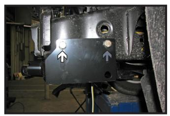
8. With the baseplate as a template, use a 17/32" drill bit to drill the two (2) holes on the sides of the baseplate. Insert a 1/2"-13 x 1-3/4" hex bolt, 1/2" lock washer and 1/2"-13 nylon hex nut into the front hole (white). Then insert a 1/2"-13 x 1-3/4" bolt, 1/2" lock washer and 1/2"-13 whiz nut plate into the back hole (gray).
