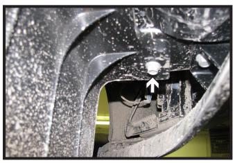
4. **2010-11 Models:** Using a 13MM socket, remove the lower air dam from the vehicle. The air dam will not be reinstalled.
