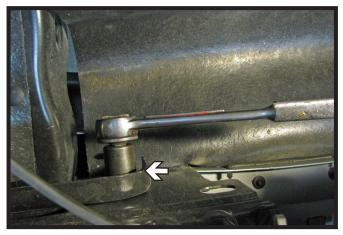
From the top side of the bumper, using a 21MM socket, remove the bolt from inner side of the frame. Do this on both sides of the vehicle.
