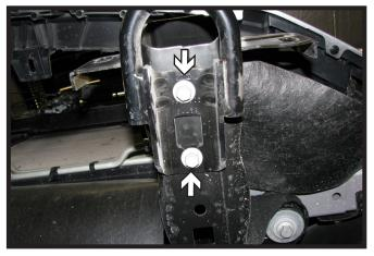
Remove the tow hook from both sides by removing the two bolts using a 15MM socket. Set tow hooks and bolts aside, they will not be reinstalled.
