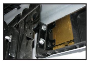
10. Install the electrical bracket on either side of the vehicle depending on the location of the plug in of the coach. Hold up the bracket and mark on the back side. Attach with 1/4"-20 x 3/4" hex bolts, 1/4" lock washers, 1/4" flat washers and 1/4"-20 whiz nuts.
