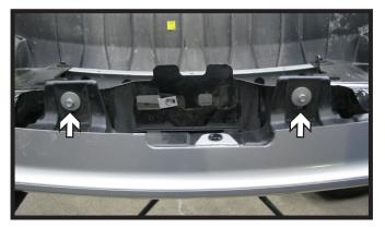
Using a 8MM socket, remove the two (2) bolts from the top side of the bumper.
