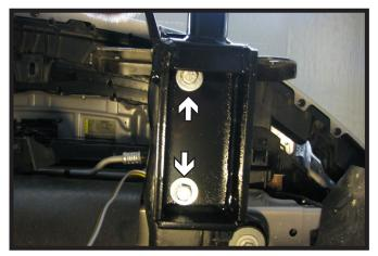
6. Hold the baseplate up, align with the existing two (2) holes on the bottom of the frame. Insert 1/2"-13 x 1 3/4" bolts, 1/2" lock washers and 1/2" flat washers. Do this to both sides.
