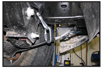
9. Attach the permanent baseplate safety cables to the provided convenience link on the baseplate. The photo above shows the recommended installation of the cables to frame of vehicle. Additional options may interfere with suggested mounting; in this case, secure the cables to a solid piece of the frame as described in the instructions included with the permanent baseplate safety cables. Be sure the safety cables do not rub against any hoses or moving parts. Do this on BOTH sides of the vehicle.
