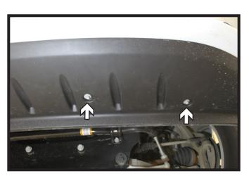
Using a 10MM socket, remove the four (4) screws from the front spoiler. There are two (2) on each side.
