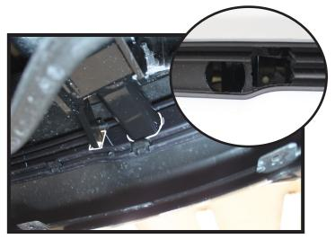
Temporarily reinstall the front cover. Hold the baseplate up as close to its installed position. Mark the backside of the front cover. Remove and trim the cover to allow the baseplate to pass thru. Do this on both sides of the vehicle.
