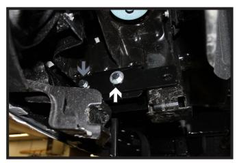
9. Bolt the side plate to the baseplate with a 1/2"-13 x 1-1/2" bolt with 1/2" lock washer and a 1/2"-13 lock nut into the front hole (gray) and a 1/2"-13 x 1-1/2" bolt with 1/2" lock and flat washers into the middle hole (white). Tighten all fasteners. Do this on both sides of the vehicle.
