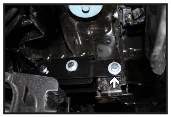
10. Using a 17/32" drill bit, drill the rear side plate hole thru the tow hook bracket. Install a 1/2"-13 x 1-1/2" bolt with 1/2" lock and flat washers into the hole with 1/2" nut wires on the inside of the bracket and tighten. Do this on both sides of the vehicle.
