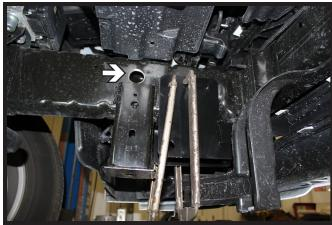
6. Clamp the baseplate into position. Using a 1-1/4" hole saw, drill an access hole above the tow hook bracket on the inside of the frame. Do this on both sides of the vehicle.
