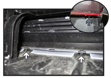
2. Remove the seven (7) push pins (white) and the two (2) plastic rivets (gray) from the inside edge of the spoiler where it meets the bumper. Set the spoiler aside.
