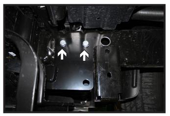
8. Using a 17/32" drill bit, drill the upper two (2) holes of the baseplate thru the frame. Install 1/2"-13 x 1-1/2" bolts with 1/2" lock washers into the holes with 1/2" nut wires on the inside of the frame and tighten. Do this on both sides of the vehicle.
