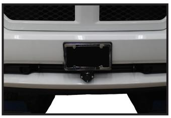
14. The electrical connection can be mounted in several locations with a combination of different hardware to suit the users need. Shown above is using the electrical bracket attached to the bottom of the license plate bracket.
