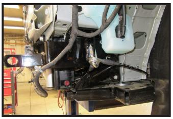
19. Attach the permanent baseplate safety cables to the provided convenience link on the baseplate. The photo above shows the recommended installation of the cables to frame of vehicle. Additional options may interfere with suggested mounting; in this case, secure the cables to a solid piece of the frame as described in the General Information sheet. Be sure the safety cables do not rub against any hoses or moving parts. Do this on **BOTH** sides of the vehicle.
