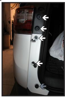
1. Remove the covers for the five (5) bolts on the back panel of the vehicle. Then using a 7MM socket, remove the four (4) top bolts (white) and a T20 Torx socket to remove the one (1) bottom bolt (gray). Do this on both sides of the vehicle.
