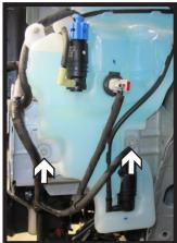
7. On the driver side of the vehicle, using a 10MM socket, remove the one (1) nut from the top of the windshield washer fluid reservoir. Disconnect all lines. Then using a 10MM socket, remove the two (2) bolts at the bottom of the reservoir.
