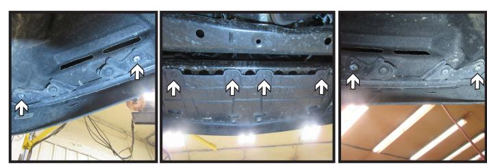
5. Using a T15 Torx, remove the eight (8) bolts from the underside of the fascia. There are two (2) on each side and four (4) in the middle.
