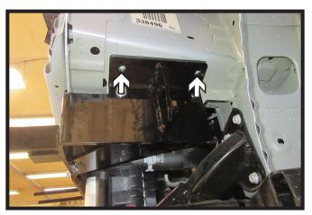
15. Using a 3/8" drill bit, drill the top two (2) holes. Install 3/8" hardware. Do this on both sides of the vehicle.
