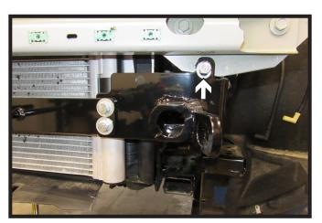
17. Using a 3/8" drill bit, drill the one (1) hole on the front of the bumper. Install 3/8" hardware. Do this on both sides of the vehicle.
