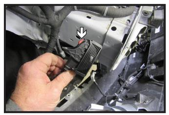
6. Start to remove the fascia. As the fascia is removed unplug the temperature sensor on the passenger side by pressing down on the red button and then pulling down on the handle to disconnect plug from sensor. Remove fascia and set aside to be reinstalled later.
