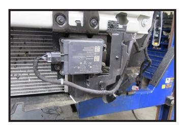
Unsnap the Adaptive Cruise Control (ACC) wire loom from the shutter housing and bumper on the driver side of the vehicle.
