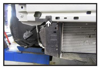
Using a 7MM socket, remove the two
