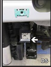
11. Using a reciprocating saw, trim the brackets on the driver and passenger sides of the vehicle as indicated to allow clearance for the baseplate.
