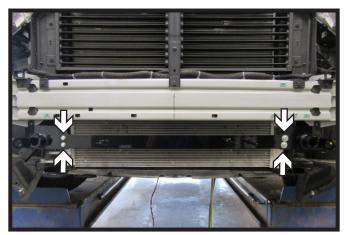
14 . Install the cross bar using four (4) 3/8" bolts, two (2) on each side, with lock washer and two (2) flat washers in between the side bracket and cross bar for each bolt as a spacer.
