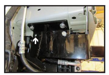
16. Using a 3/8" drill bit, drill the one (1) back hole. Install 3/8" hardware. Do this on both sides of the vehicle.
