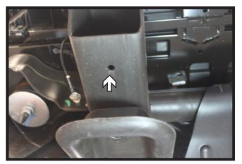
6. Using a 17/32" drill bit, drill out the existing hole in the bottom of the frame. Do this on both sides of the vehicle.
