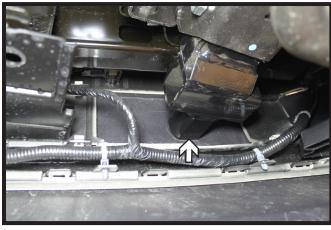
Partially reinstall the fascia with a couple of screws along the top and pull the fascia tight
