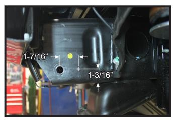
7. Using a 17/32" drill bit, drill a hole thru the frame 1-7/16" back from the existing hole and 1-3/16" up from the bottom of the frame. Do this on the outside driver side frame and the inner passenger side frame. (Driver side shown)
