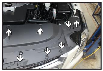
1. Remove the fourteen (14) push pins from the fascia cover and set aside. There are seven (7) on each side.
