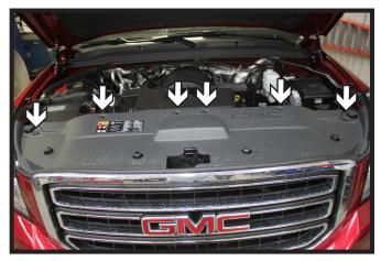
Remove the six (6) push pins from the fascia cover and unsnap the front edge. Set the cover aside.
