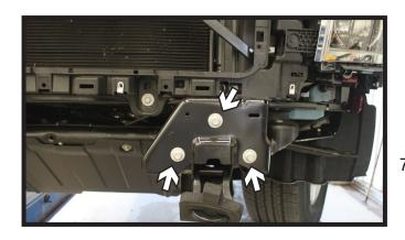
7. Using a 15MM socket, remove the three (3) bolts from the cover plate. Do this on both sides of the vehicle.
