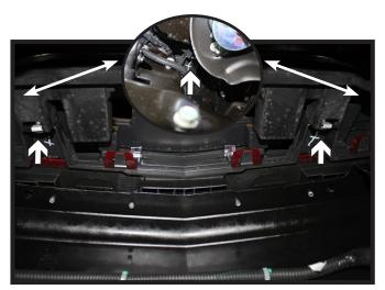
Using a 10MM socket, remove the four (4) screws from the underside of the fascia.
