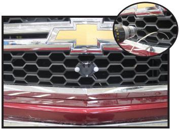
13. **Optional:** Prior to fully reinstalling the fascia. Using a 1/4" drill bit, widen the grille opening to accommodate the plug bolts. Using 1/4" x 1-1/2" bolts with 1/4" washers, install the plug thru the grille. On the backside of the grille, install the electrical bracket and 1/4" locknuts to secure the plug to the grille.
