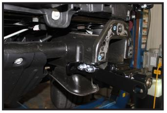
10. Position the appropriate baseplate into the tow hook pocket. Install 1/2"-13 x 5" bolts from the outside of the frame with the convenience link, 1/2" lock washers and lock nuts on the inside of the frame. Tighten down until the frame squeezes against the baseplate. Do this on both sides of the vehicle.
