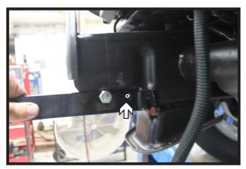
9. Place the convenience link against the frame and pin the front hole with a 1/2" bolt. Level the link and mark the frame for the rear hole. Do this on the inside passenger and outside driver frame rails. Using a 1/2" drill bit, drill out both holes to line up with the existing holes on the other side of the frame.
