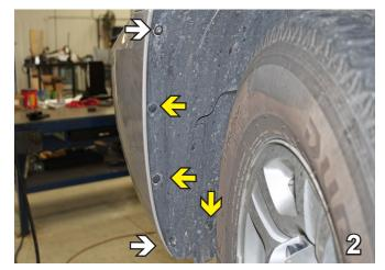
In front of the tire, remove two bolts with a 7MM socket (white arrows). Using a flat screwdriver, remove three push pins (yellow arrows). Do this to both sides of the vehicle. Set bolts and push pins aside to be reinstalled later.
