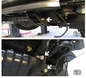
Using a 18MM socket, remove one bolt from the side and one bolt from the bottom of the tow hook. Do this to both sides of the vehicle. Factory tow hooks and bolts will not be reinstalled.
