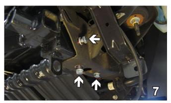
Slide baseplate in where the tow hooks were removed. Insert a 1/2-13 x 1-1/4" hex bolt with Loctite Red and 1/2" lock washer into the two (2) holes on the side and the two (2) holes on the bottom of the baseplate and tighten bottom two (2) bolts down first. Do this to both sides of the vehicle.
