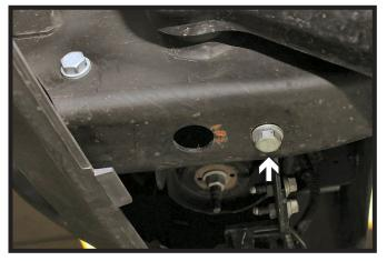
1. Using an 18MM socket, remove the three (3) bolts from the tow hook. Pull tow hook forward and set aside. Tow hooks will not be reinstalled. Do this on both sides of the vehicle.
